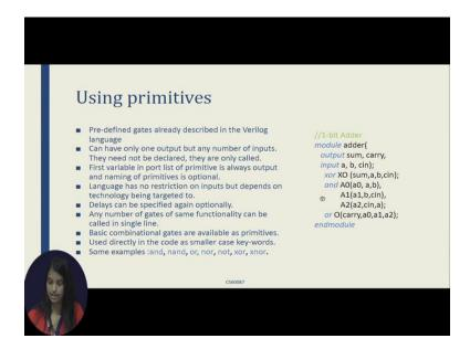
So, we saw how we use predefined gates earlier in structure modeling, so we call them primitives. So, if you can see here I have taken an example of adder this is a 1 bit adder I have taken which has a sum and carry out put two in three inputs a b and c.
