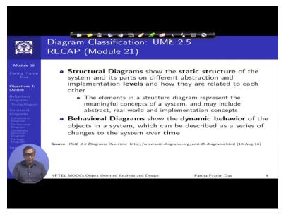
So just to remind you the structural diagrams of the uml, so the structure of the system and parts of different abstractions at a level and a behavioral diagrams show the dynamic behavior basically showing you how does a system behave over a time.
