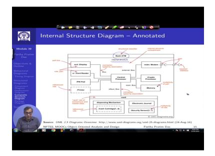
Let us quickly go to an example. so here we are talking about a bank ATM and this is we are trying to show the internal structure. So in terms of the internal structure now you can see what does a you are trying to describe now the internal structure of an automatic teller machine. So it must have a display obviously, it must have a card reader where you put the card, it must have a key board being paired so that it can key in the print.
