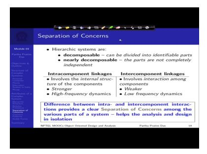
The next is, the next attribute of complex system is separation of concerns that is hierarchic systems are decomposable that is what we have seen then they can be divided into identifiable parts, personal computer decomposable in terms of CPU, hard disk, monitor, keyboard, and so on. At the same time, interestingly they are nearly decomposable in the sense that while we say that these are all decomposable but they are not completely independent.
