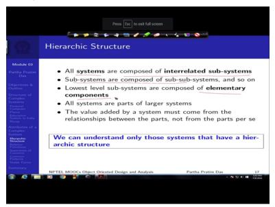
And we have also taken a brief look into hierarchic structure that is we say that every system is composed of interrelated subsystems and sub-sub systems till you go to an elementary component level. This is a basic property that we say will exist in any complex system that we analyze.
