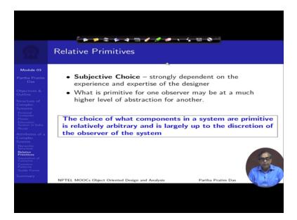
Now next is relative primitive that is if we keep on decomposing the system in the hierarchy manner as we have said and then there are some where you will have to stop and that stopping point is called the relative primitive or the primitive. It is relative because there is, there cannot be a unique definition of what is a primitive. It is a matter of perception of the observer of the designer as to deciding what is a primitive.
