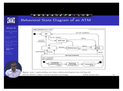
So given this is the behavioral state diagram of an atm. I will not go through the details, we have just briefly discus this and I will request that you please go through each of these state transitions and get comfortable in terms of describing an atm system to this kind of an fsm.
