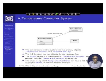
So we will just take a look into a couple of simple examples. Here is one, example of a temperature controller which has three objects certainly this one; the first one is the controller which decides to maintain a certain temperature profile for an industrial process. The temperature profile that needs to be maintained use an object itself which we say is a temperature ramp that is how the temperature should increase, how should it decrease and so on.
