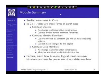
So, with this we come to the end of the current module. Here we have studied const-ness in C++, in C++ we have seen three forms of const-ness, the object as a whole can be constant and if the object is constant, then it can only invoke constant member functions.
