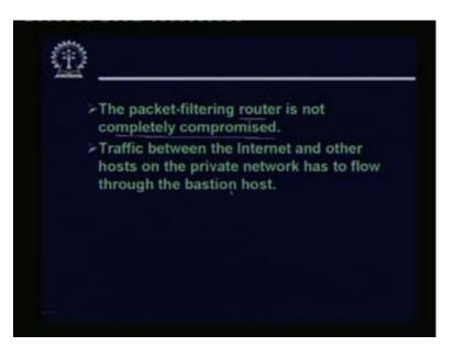
So here the packet filtering router. You cannot completely compromise the system by compromising that. So now all traffic between internal and outside network has to flow through the bastion host. This is one very important characteristic out here. Now let us go one step further.
