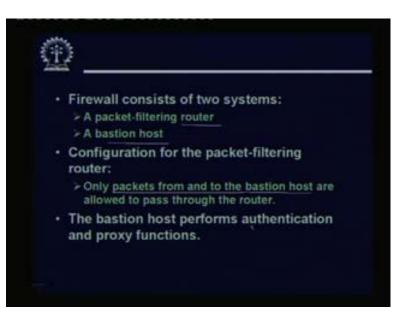
So as we have seen that in this method the firewall consists of a router and a bastion host. So the router as I said it will only allow packets to and from the bastion host to flow. The bastion host can perform authentication. It can also perform the proxy functions.
