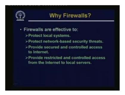
Firewalls we use to primarily locate to protect our internal network to protect the local systems which are there as part of our own network. Protect against several network based security threats. There are so many published kinds of security breaches and threats
