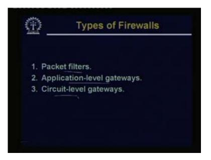
Broadly speaking there are three types of firewalls we encounter. Firewalls based on packet filtering mechanism. Based on application level gateways, based on circuit level gateways, let us try to see what these are.
