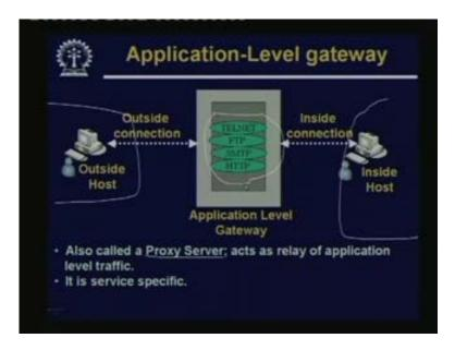
And these rules are the techniques which you are filtering will be very much service specific. This basically acts as a relay of application level traffic and it is service specific.
