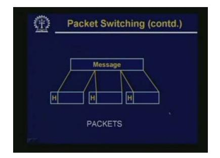
So this diagram shows how a message can be broken up into packets. A message gets broken up into 3 packets and each packet will be having its own header. This header will allow this packet to reach the destination and to have the intermediate nodes take the appropriate decision to route the packets accordingly.
