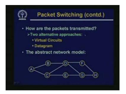
Now regarding the mode or the way the packets are transmitted, there are two alternate approaches. These are called virtual circuits and datagram. The abstract data model will be same as I had shown earlier. So there will be a number of nodes ABCDEFGH which will be connected by links and the main responsibility of the packet switching will be to send the data from some nodes, say A to a destination say H, this will be main responsibility.
