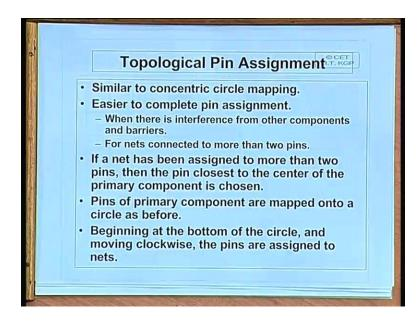
See topological pin assignment is similar. So see in case of concentric circle mapping you are assuming that there are that there are no abstractions in between. When you are trying to interconnect you have finding the shortest distance. But topological pin assignment assumes that there can be some abstractions or interference from other components which can act as barriers. So you will have to go around the barriers for interconnections. So the idea is like this.
