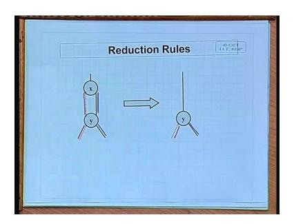
The first reduction rule is this. It says that if in the graph you have 2 nodes like this where these are the negative edges or the dotted lines these are the positive edges, then if from a node both negative and the positive edge is leading to the same node in the second level. Then you can omit
