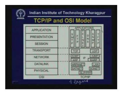
Although the TCP/IP was developed much earlier than OSI model always we try to map a particular protocol with the OSI model. Let us see what is the relationship between the TCP/IP and the OSI model.
