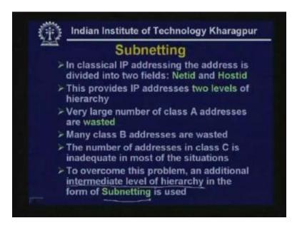
This problem can be avoided by introducing an intermediate level of hierarchy in the form of subnetting. So what is being done is in subnetting the addresses the addresses divided into three parts; the net ID, subnet ID and the host ID as it is shown here.
