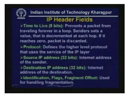
Then the source IP address is necessary which is 32-bits the destination IP address and this identification, flags and fragment fields are used for the purpose of fragmentation.
