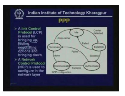
This is the flow diagram for PPP protocol. Apart from using this HDLC framing it sets up the link with the help of Link Control Protocol LCP so it uses for bringing up testing and negotiating options and also for bringing down.
