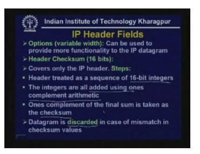
There is other options field, this can be used to provide more functionality to the IP datagram and there is a checksum field which is of sixteen bits. Checksum is done only for the header part so header is treated as sixteen bit integers, the integers are all added using ones complement arithmetic, then the ones complement of the final sum is taken as the checksum and if the checksum does not match then the frame is discarded.
