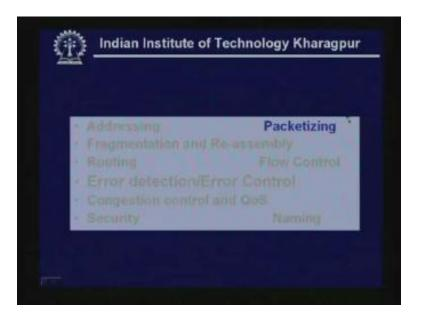
Now let us consider the second issue that is packetizing. Packetizing means the data has to be sent in a format of frame and the packet is used by the internet protocol to frame a datagram or frame. So the datagram includes the header comprising a number of fields and apart from data it adds a header. The header has a number of fields as explained here.
