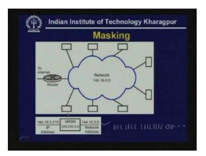
Now you may be asking whenever an IP address is being used how a particular network receives a particular packet which is made for that network, this is done with the help of a technique known as masking.
