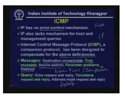
Redirect message: this is necessary. Whenever a router receives a packet it is not made for that particular router. So it redirects it towards the proper destination at the same time it informs the source about the redirection. These are the various messages that is being supported by ICMP.
