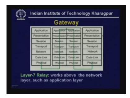
Finally this is the gateway as I mentioned which works above the network layer such as application layer. So here you see the gateway operating in application layer and two
