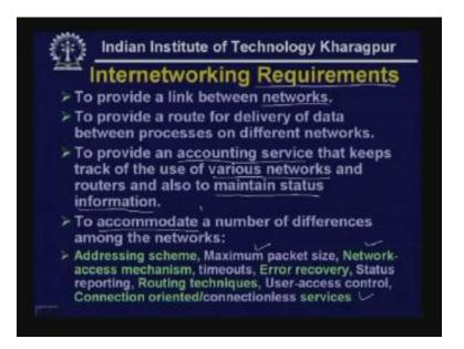
So let us have a look at the various requirements for internetworking. First objective is to provide link between networks. You have got isolated networks, LANs and WANs you would like to link them together and link between these networks to provide a route for delivery of data between processes on different networks. That means processes running on different networks has to be provided a route so that from one network it can be transferred or delivered in another network.
