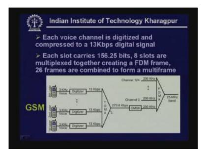
This (Refer Slide Time: 42:43) generates 200 KHz analog signal which is sent to the transmitter from the mobile station to the base station. Similarly, from the base station to different mobile stations it is sent except the carrier frequencies will be different. So you have got 124 channels so each of these channels can support eight different users sending digital voice or digital data which is also possible. This is how communication is performed in GSM.
