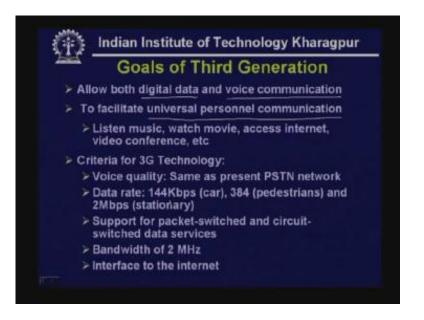
The third generation technique uses both digital data and voice communication. So, in case of your second generation either voice or data of very low capacity can be sent. But here the objective is to send data of little higher rate and good quality voice. And one objective is to provide universal personal communication that means one can listen to music, one can watch a movie, one can access the internet so all these things are possible by using third generation technique.
