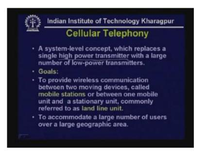
It is essentially a system level concept which replaces the single high power transmitter with a large number of low power transmitters. Conventionally a very high power transmitter is used when a large geographic area is used to be covered. But this concept is not used in cellular telephony or cellular telephone networks.
