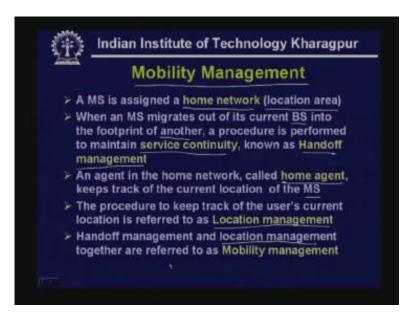
As you have already seen a mobile station is assigned a home network over which it can roam around and which is under the control of a mobile switching center called as the location area. When a mobile station migrates out of the current base station into the footprint of another a procedure is performed to maintain service continuity. This is known as handoff management. How it is been done?
