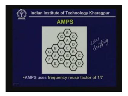
Now in case of second generation communication it was based on digital technique. We have seen AMPS uses analog communication and it is very easy to perform eavesdropping. That means any receiver receiving a particular carrier frequency or when the channel is tuned to that particular frequency then it will be able to receive the voice.
