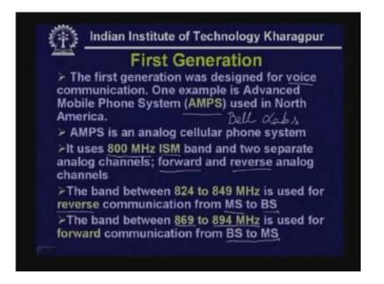
On the other hand the band between 869 to 894 MHz is used for forward communication from base station to mobile station. Let's see pictorially how it operates.
