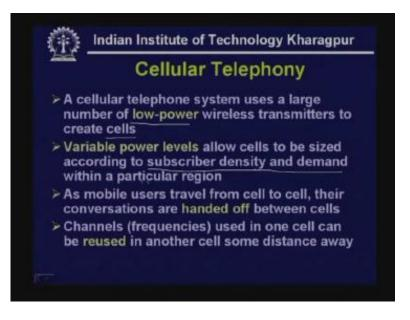
As mobile users travel from cell to cell their conversations are handed off. That means when a user or a mobile station moves from one place to another it is very common that they will move away from a particular cell and go to a new cell so it has to be done in a seamless manner and the approach to be used to satisfy seamless transfer is known as handoff. So, the conversation is to be handed off between cells.
