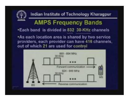
These are two different bands, this (Refer Slide Time: 26:20) is for forward communication 869 to 894 mega band divided into 832 30 KHz channel so you have got 832 30 KHz channel distinct channels with different carrier frequencies and similarly for reverse communication from the mobile station to the base stations you have got again 832 frequency bands each of 30 KHz.
