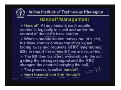
As we have seen at any instant each mobile station is logically in a cell and under the control of cell's base station. Now, when a mobile station moves out of a cell the base station notices mobile station's signal fading away and it requests the neighboring base stations to report the strength they are receiving. The base station then transfers ownership to the cell getting the strongest signal and the mobile switching center changes the channel carrying the call.
