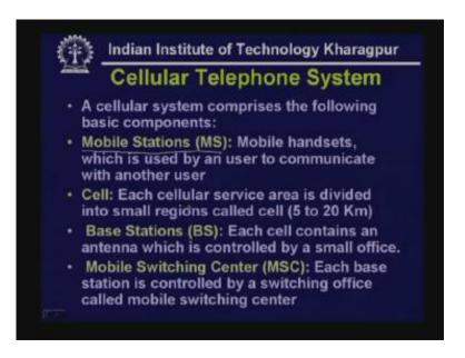
And there are base stations; each base station contains an antenna which is controlled by a small office. In addition to that there is mobile switching center where each base station is controlled by a switching office called mobile switching center, it will be clear from the next diagram.
