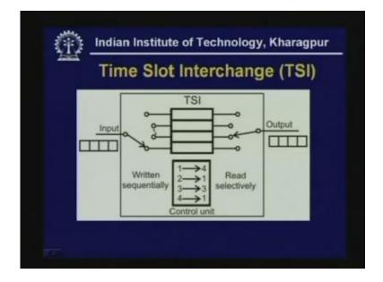
So here you can see the data is coming in slots then it is stored in some memory so in this memory the writing is done in a sequential manner that means 1 2 3 4 and then reading is done selectively. That means here the writing takes place sequentially and reading takes place sequentially that's how the Time Slot Interchange takes place and data goes from 1 to 4, 2 to 1, 3 to 3 and 4 to 1. This is how it takes place in Time Slot Interchange.
