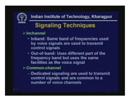
On the other hand the common channel is dedicated signaling are used to transmit control signals and are common to a number of voice channels. So we have discussed by the circuit switching technique and it is time now to give you review questions. Here are the five review questions.
