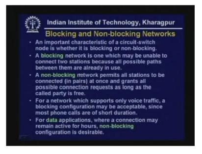
Let me introduce the concept of blocking and non-blocking before I discuss the other functions of the cross bar switch. An important characteristic of a circuit switch node is whether it is blocking or non-blocking.
