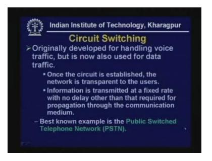
Now let us look at the advantages of this circuit switching technique. First it is fixed bandwidth and guaranteed capacity. That means there is an end-to-end link and since end-to-end link is there the bandwidth is fixed and it does not change.
