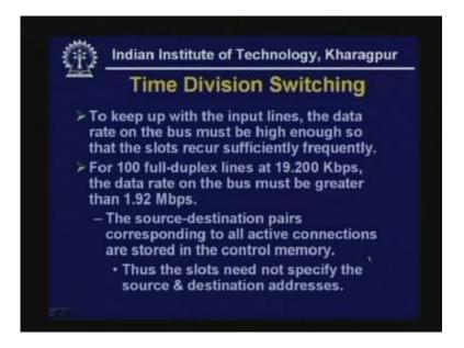
So here for example we have a simple TDM where the switching is not done.
