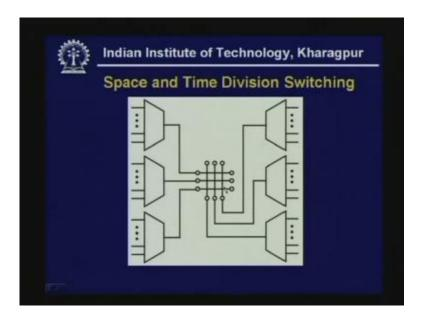
However, you can combine the space and Time Division Switching. we have already discussed the Space Division Switching and Time Division Switching and it can be combined here. So these are the typical TDM switches Time Division Switches and here it is Space Division Switches which is nothing but a crossbar. Therefore as you can see here this interchange can be done with the help of this crossbar switch.
