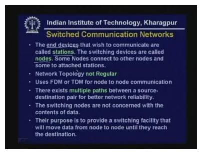
In switched communication network we will find end devices namely essentially computers, peripherals, communication equipments such as cell phones, laptops PDAs and various other things and these are known as stations. The switching devices are called nodes. That means we are using some additional devices intermediate devices known as nodes and in such a situation some nodes connect to other nodes and some nodes are attached to stations. Let me show you the network.
