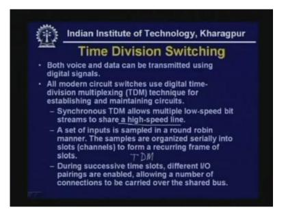
We have already discussed about TDM or Time Division Switching which is essentially based on Time Division Multiplexing and here both voice and data can be transferred using digital signals and all modern circuit switches use digital Time Division Multiplexing techniques for establishing and maintaining circuits and synchronous TDM allows multiple low speed bit streams to share a high speed line. We shall explain how exactly this is being done.
