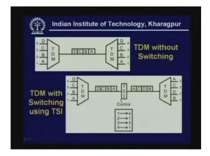
So in this case it is 1 2 3 4 where 1 is sending in data in slot A, 2 is sending in slot B, 3 is sending in slot C and 4 is sending slot D and slot A is again taken to 1 and slot B data goes to 2, slot C data goes to 3 and slot D data goes to.... this is the simple Time Division Multiplexing. Obviously this will not serve our purpose so we have to use something in between. The first thing that can be done is TSI. TSI stands for Time Slot Interchange.
