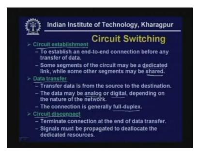
Then in data transfer the transfer data is from the source to the destination. Once the link is established whatever data is to be transferred is transferred from the source to destination through the dedicated link already established in that circuit establishment phase. then the data may be analog in nature or digital in nature either is possible depending on the nature of network and the connection is generally full-duplex.
