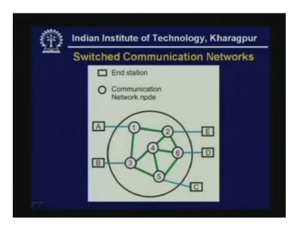
Here as you see these are the end stations A B C D E and on the other hand 1 2 3 4 5 6 are communication networks nodes so these are the nodes used as switches as
