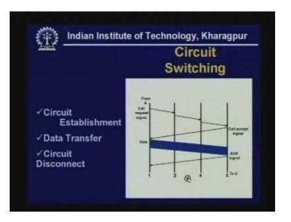
This circuit switching technique was originally developed for handling voice traffic but is now also used for data traffic.
