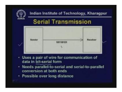
As you can see in serial transmission a pair of wire is used for communication of data in bit serial form. Instead of sending in parallel you are sending it bit by bit. As you can see here we are sending them one by one, first one, then 0, then 1, then 0, then 1 and 0 and 1 and 0 and 1 so in bit serial fashion and of course this will require parallel to serial conversion by the sender and also it will require serial to parallel conversion at the receiving end (Refer Slide Time: 8:00).
