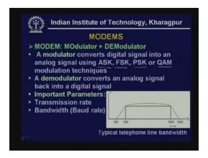
Here there are two important parameters as you know the transmission rate and the baud rate. Here are the various baud rate and data rate is explained based on different modulation techniques. As you have seen using smaller baud rate we can achieve bit rate or data rate.
