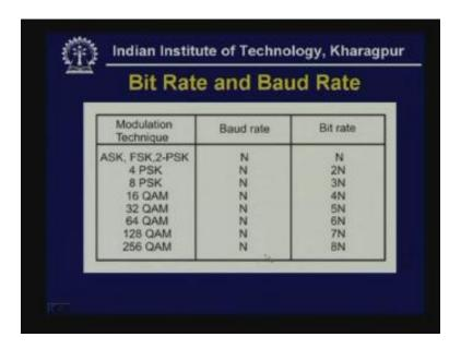
If we use 256 QAM it can be eight times, for example if we are using the typical telephone line having the bandwidth of 2400 that is the baud rate so we can multiply it by 8 if we use 256 QAM that will be data rate. So 8 into 2400 can be the data rate in this particular 256 QAM. And some modems have been developed by ITUT and Bell laboratories. The modems developed by Bell laboratories are known as bell modems and ITUT developed modems are V series modems.
