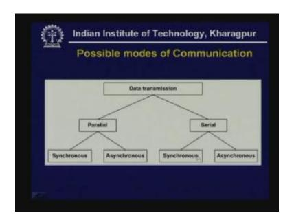
Data can be transmitted in parallel or in serial. Again parallel has two different types synchronous and asynchronous and serial also has two variations synchronous and asynchronous. First let us consider the Parallel Transmission technique.
