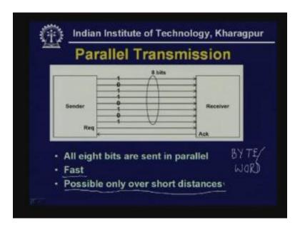
In Parallel Transmission technique as you can see a number of bits usually a byte or a word it can be either a byte that is 8-bit or it can be word. Word can be 8-bit, 16-bit, 32-bit or 64-bit depending on the size of the processor it can be byte or word that is sent in parallel. As you can see all the bits are transmitted parallel between the sender and receiver. Obviously whenever you transmit data in this manner it is very fast because all the bits are going simultaneously.
