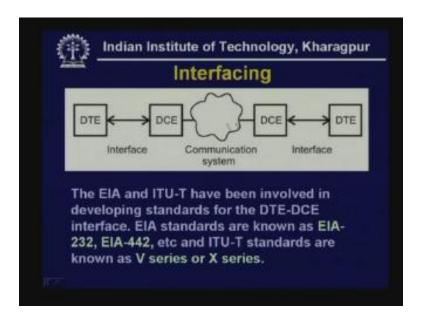
Therefore DCE is usually the modems. The DTEs are computers and various other equipments that we use for sending data. Now the interface has to be universally accepted so that the two equipments one DCE and another DTE manufactured by two different companies can be interfaced. For that purpose some standards are to be used. The standards are developed by two organizations the EIA Electronic Industries Association and ITUT or the DTE DCE interface.
