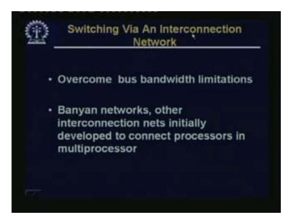
Switching via an interconnection network are just as in the other kind of switches we have seen. It overcame bus bandwidth limitations, that is the basic implication. As we want to go faster and faster, we have to migrate from buses to an interconnection network. We have already seen Banyan networks. Other interconnection was initially developed to connect processors and multiprocessors, etc. It became useful in this class of packet switches.
