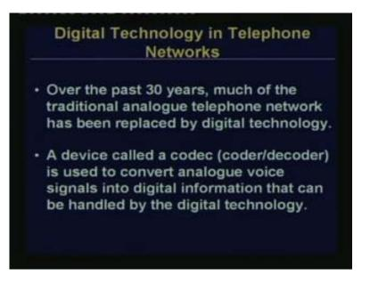
Now we will take a quick look at the digital technology in the telephone network. As mentioned earlier, traditionally everything was analog. Then the exchanges started getting converted to digital technology, so a device called a codec is used to convert analog voice signals into digital information that can be handled by digital technology.
