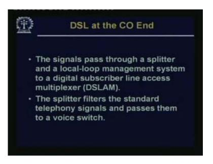
So with DSL at the central office end, CO end, the signals pass through a splitter as I have shown and a local loop management system, so the subscriber line access multiplexer is there.
