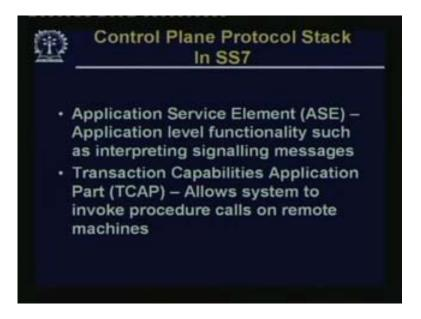
So these are some of the elements which are there in SS 7: application service element, that is application level functionality such as interpreting signaling messages, then the transaction capabilities, which allow systems to invoke procedure calls on remote machines, Signaling connection control part SCCP, connections, sequence numbering, segmentation, reassembly, flow control, etc. Some of these terms may not make any sense at the moment so we will discuss this later on in other context.
