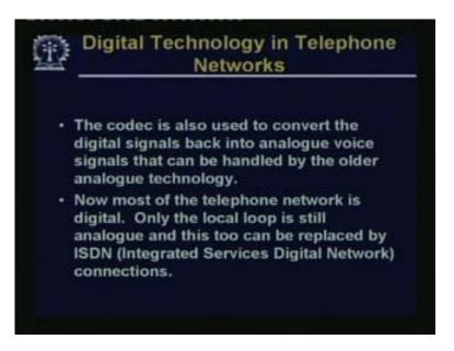
The codec is also used to convert the digital signals back into analog on the other side, so that voice signals that can be handled by the older analog technology. Now most of the telephone network is digital; only the local loop is still mostly analog.
