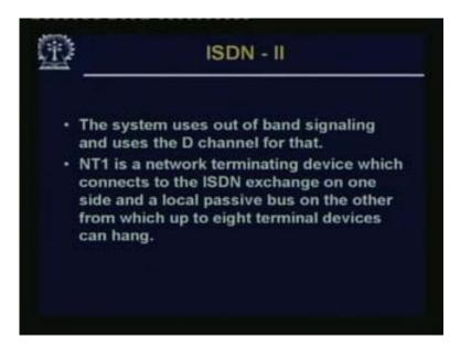
The system uses out-of-band signaling and uses the D channel for that. NT1 is the network terminating device, which connects to the ISDN exchange on one side and a local passive bus on the other.
