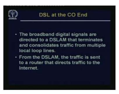
The broadband digital signals are directed to a DSLAM that terminates and coordinates traffic from multiple local loop lines, from the DSLAM the traffic is sent to a router and then to the internet. And finally we have the loop management system; this may be in front of the splitter or behind the splitter.
