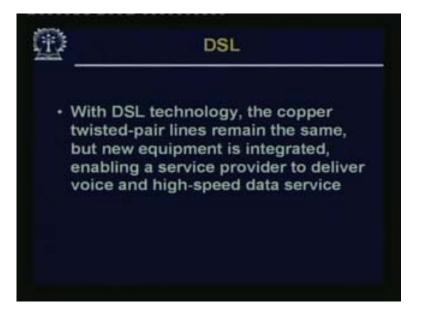
The copper twisted pair remains the same, but the new equipment is integrated, enabling a service provider to deliver voice and high-speed data service at the same time. So this is the picture that shows subscribers who are connected through the analog and DSL lines. Now in the centre of the side, you have some kind of a splitter and in this splitter, one side is the data: (Refer Slide Time: 54:20)
