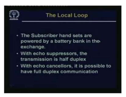
Local loop: The subscriber handsets are powered by a battery bank in the exchange. For example, I mean with at least the ordinary handsets, you do not need to connect it to any power; it actually derives its power from the same cable which is coming and connecting your telephone set. And with echo suppressors, the transmission is half duplex and with echo cancellors, it is possible to have full duplex communication.
