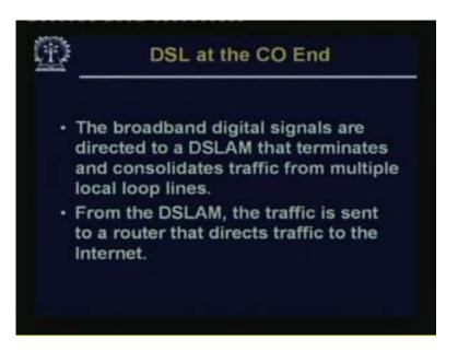
From the DSLAM, the traffic is sent to a router and then to the internet. And finally we have the loop management system, which may be in front of the splitter, or behind the splitter?
