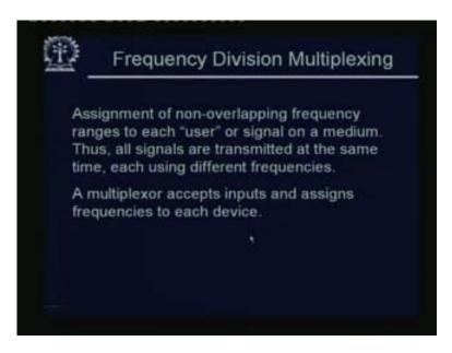
These systems all use frequency division multiplexing. This technique is the oldest of the multiplexing techniques. Assignment of non-overlapping frequency ranges to each user or signal on a medium –all signals are transmitted at the same time, each using different frequencies. A multiplexer accepts inputs and assigns frequencies to each device.
