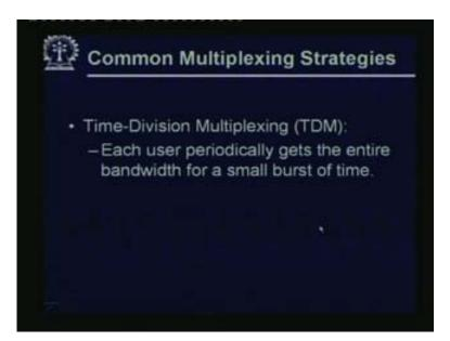
Just quickly before we get into the details of each of these, in time-division multiplexing, each user periodically gets the entire bandwidth. That means the entire channel is dedicated to one user but only for a short period of time, for a small burst of time. After that it is somebody else's time. We will look at the details of this later.
