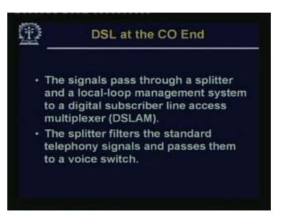
So DSL at the central office end, CO end, and the signal passes through a splitter as I have shown and a local loop management system. The subscriber line access multiplexer is there in this figure we have already seen. (Refer Slide Time: 57:39)
