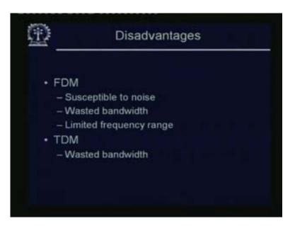
Just a quick look at the disadvantages: FDM, as I mentioned earlier, is susceptible to noise, wasted bandwidth, because of this guard band, etc., and of course one frequency is whatever the small band is being permanently given to one user and if his usage is very bursty, then a lot of bandwidth is wasted. Then, we have a limited frequency range. In TDM we have wasted bandwidth for the same reason.
