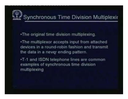
The synchronous time division multiplexing, remember that it is synchronous because the multiplexer and the demultiplexer has to agree about the slot of time; the original time division multiplexing, the multiplexer accepts input from attached devices in a round robin fashion and transmit. T1 and ISDN telephone lines are common examples of synchronous time division multiplexing.
