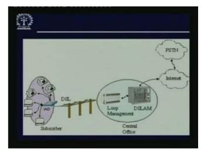
In this figure, we have DSLAM and the loop management over there, the broadband digital signals is directed to a DSLAM that terminates and coordinates traffic from multiple local loop lines.
