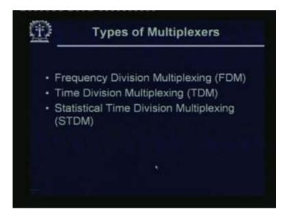
The types of multiplexer we have are: FDM, that is, frequency division multiplexing; TDM, that is, time division multiplexing; STDM, that is, statistical time division multiplexing. We will look at these.
