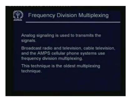
Usually for frequency division multiplexing, analog signaling is used to transmit signals. Broadcast radio and television, cable television and amps cellular phone system use frequency division multiplexing. Amps are an old cellular phone system that was there in USA. Nowadays of course, the kind of Cellular technology that we have in our country uses more complex multiplexing techniques; maybe I'll mention that later on.
