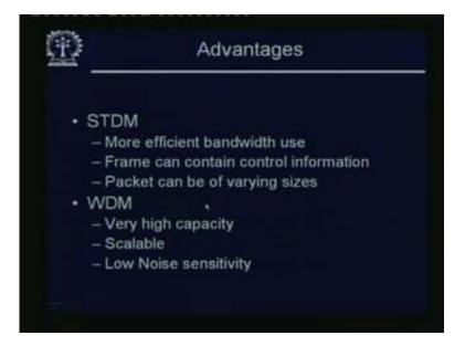
STDM's advantages: we are only talking about advantages. We will talk about disadvantages later on. In statistical time division multiplexing, this has certainly more efficient bandwidth use. It is much more efficient because as I mentioned, that especially data usage and usage in general may be very bursty and if it is bursty, then during the quiescent period, ordinary TDM is just wasting the channel whereas STDM is making full use of it.
