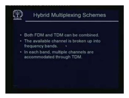
In hybrid multiplexing system, both FDM and TDM may be combined; the available channel is broken up into frequency bands; in each band multiple channels are accommodated through TDM.
