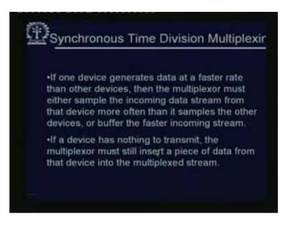
If one device generates data at a faster rate than other devices, then the multiplexer must either sample the incoming data stream from that device more often than it samples the other devices or buffer the faster incoming stream. If a device has nothing to transmit the multiplexer must still insert a piece of data from that device into the multiplexed stream, it may be a dummy data.
