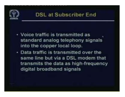
So DSL at subscriber end- voice traffic is transmitted as standard analog telephony signals; data traffic is transmitted over the same line via a DSL modem that transmits the data as high frequency digital broadband signals on the same line. If you have DSL modem you can have both your voice as well as data at the same time, unlike very ordinary analog lines.
