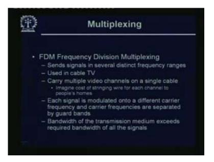
The bandwidth of the transmission medium exceeds required bandwidth of all signals because of these guard bands which have to come in-between.
