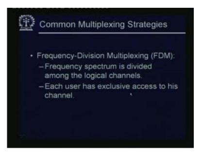
Another common approach is the frequency division multiplexing; here the frequency spectrum is divided among the logical channels. Here we have only one physical channel, but we want to have a number of logical channels, so the frequency spectrum of the channel is divided, each user has exclusive access to his channel.
