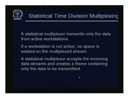
To summarize, a statistical multiplexer transmits only the data from active work stations. If a work station is not active, no space is wasted on the multiplexed stream; a statistical multiplexer accepts the incoming data streams and creates a frame containing only the data to be transmitted and also as I said this frame will also contain the some kind of destination address.
