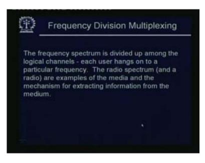
As was mentioned, the frequency channel is divided into logical channels; each user hangs on to a particular frequency, the radio spectrum and a radio is examples of the media and the mechanism of extending information from the media.
