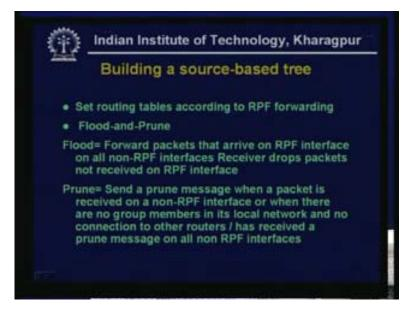
Once again that it has received on the non-RPF interface or when there are no group members in its local network and no connection to other routers or it has received a prune message on all non RPF interfaces. So in such cases the prune message is sent.
