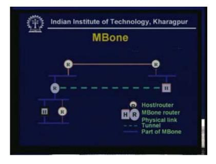
What does that mean? That means some of the routers in the network in some places are multicast-capable. And what happens is that they are going to support multicasting in its own locality. That means it will support multicasting amongst the network to which they
