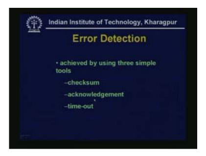
Error detection is achieved by three simple tools: Checksum, acknowledgement and timeout. Suppose you had sent the first segment and the acknowledgement never came then after sometime you have to give a time-out and that is how the sender detects that this segment has been lost and it has to be re-transmitted. (Refer Slide Time: 44:38 -44:52)
