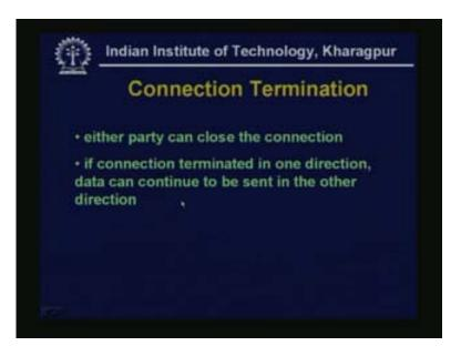
So, if connection is terminated in one direction data can be continued to be sent in the other direction.
