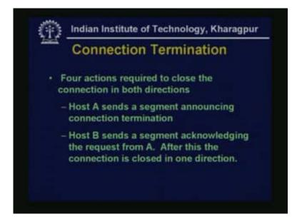
Host B sends a segment acknowledging the request from A and after this the connection is closed in one direction.
