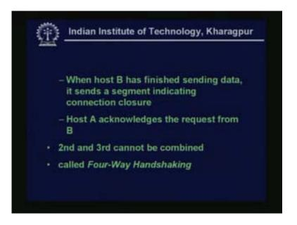
The third step can be taken only when host B has finished sending data from its side and it sends a segment indicating a connection closure. Host A acknowledges the request from B. So this is called a Four-Way Handshaking.
