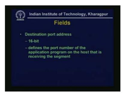
Similarly there is destination port address which is again 16-bits. The port number is from 1000 to 65000 and those are the ephemeral port numbers. Destination port address defines the port number of the application program on the host that is receiving the segment.
