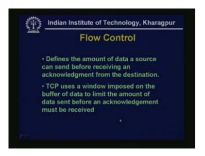
The flow control is implemented by TCP. This defines the amount of data a source can send before receiving an acknowledgment from the destination. TCP uses a window imposed on the buffer of data to limit the amount of data sent before an acknowledgement must be received. This is the traditional sliding window protocol.
