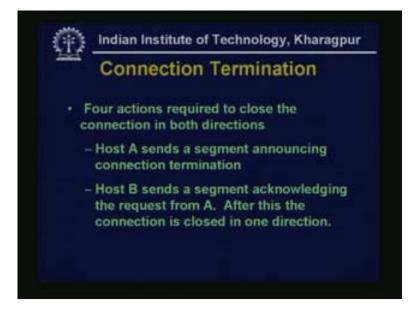
Four actions are required to close the connection in both directions. First, host A sends a segment announcing connection termination. This means it sends the segments containing FIN.
