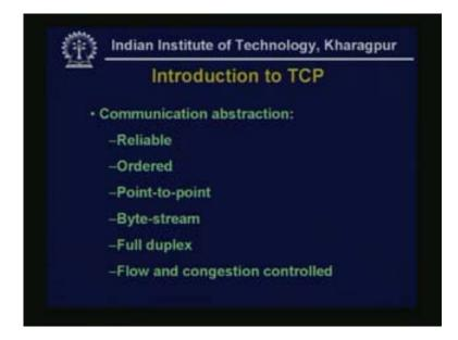
The communication abstraction is that, it is reliable and ordered. Ordered means the packets are received in order. In IP it is not guaranteed that the packets will arrive in
