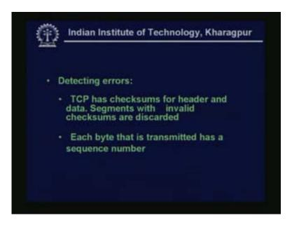
TCP can detect errors. TCP has checksum for header and data like UDP. Segment with invalid checksums are discarded. Each byte that is transmitted also has a sequence number. So, if some intermediate sequence number is missing the receiver knows that something has been lost.
