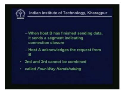
When host B has finished sending data it sends a segment indicating connection closure.
