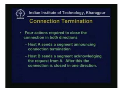
Although we are sort of allowing the termination of connection for one side but on the other side it may have acknowledgements or other things to send to this side so it will not terminate the connection. Therefore these two cannot be combined together.
