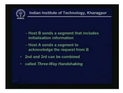
Then host A sends a segment to acknowledge the request from B. Second and third can be combined which is called as the Three-Way Handshaking.
