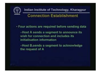
That means the host B can acknowledge the request of host A as well as in the same acknowledgement it might send the initialization information meaning the sequence number etc have to be exchanged.
