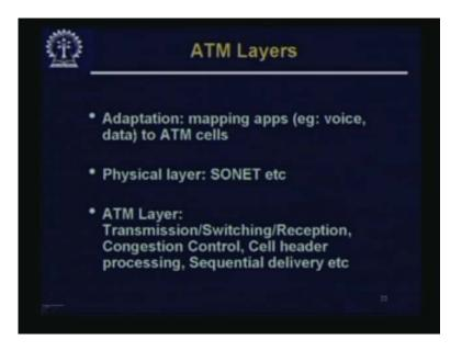
ATM layer's adaptation is mapping of application (e.g.: voice, data, etc.) to ATM cells. The physical layer could be SONET or it could simply be a DWDM system. ATM layer handles transmission/switching/reception, congestion control, cell header processing, sequential delivery, etc.
