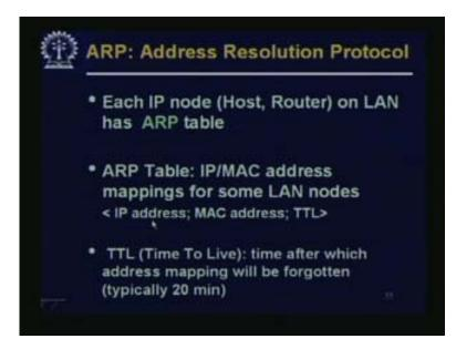
Each IP node on LAN has an ARP table. ARP table is IP, MAC address mapping for some LAN nodes. And there is a time to leave, something like 15 minutes or so, it depends on the time after which the address mapping will be forgotten – it is typically around 15, 20 or 25 minutes.
