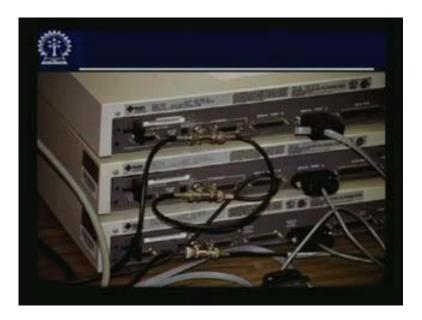
So this is the picture of hub. This is a co-axial cable coming in here and this is a t joint; the t joint is feeding into the hub. There may be a number of ports and a number of segments may be connected together.
