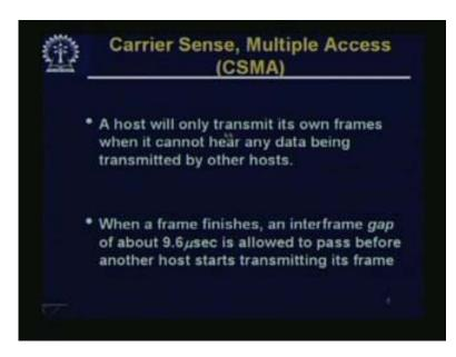
A host will only transmit its own frames when it cannot hear any data being transmitted by the other hosts. When a frame finishes an inter frame gap of about 9.6  $\mu$ s is allowed to pass before another host starts transmitting its frame. So he listens to somebody sending and then he naturally waits and then after that frame is over, he gives a gap of about 9.6  $\mu$ s and then starts transmitting Collisions can still occur mainly because of the propagation delay.
