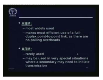
Then ABM this is the most widely used. On both sides, we have combined stations. It makes most efficient use of a full duplex point-to-point link, as there are no polling overheads. You do not have to do any polling since this is point to point. ARM is rarely used; it may be used in very special situations, whereas secondary may need to initiate transmission.
