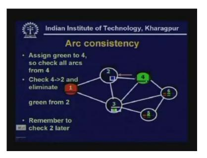
We assign green to 4. After we assigned green to 4 we check all the arcs from 4, 2, 3 and 6. First we check 2. So when we check 4 is equal to 2 we eliminate green from the domain of 2. But we have to check back later with the variables with which 2 has some constraint.
