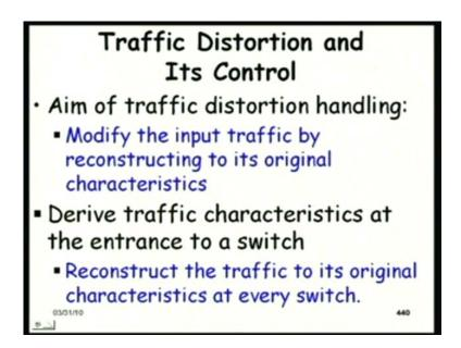
We will we will just discuss that I think in the next slide, but here just talking of the distortion handling, which we will try to reconstruct the traffic to original characteristics given that the traffic has the loose lost its shape; it has become distorted. The distortion handle mechanism will try to reconstruct the traffic. It will derive the traffic characteristics at the entrance of the switch, and reconstruct the traffic to the original characteristic that we are agreed upon.
