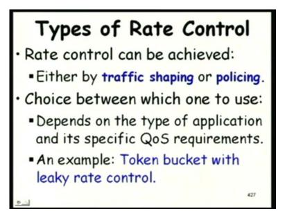
One rate control is called as traffic shaping; here, the traffic becomes out of shape, becomes busty, and then we need to reshape it to the original traffic specification; the other is policing, where we check whether the traffic meets the required characteristics for the traffic, I mean the agreed characteristics for the traffic; if not, reject it; the ones that are not satisfying reject them.
