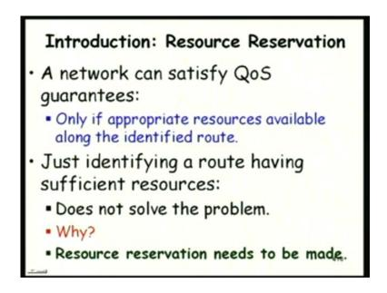
Now, once the request for a call comes, not only a path has to be established by the router, which can support the specified quality of service, but also the resources need to be reserved, because just checking whether a path exists with a specific quality of service will not guarantee that the quality of service will be met, unless it is reserved for that specific connection.
