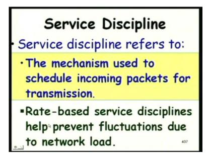
So, we can think conceptually that a service discipline is the mechanism used to schedule incoming packets for transmission. So, the packets that are incoming to a router, after the rate control is applied, they are put on the output buffer, and then they are taken up on transmission based on the service discipline. Now, we will discuss few service discipline in the subsequent slide, but one thing that we must remember is that all of them will be rate based service disciplines.
