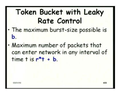
So, that is what it says the maximum burst size possible is b, and the average rate of transmission is r; r packets can be transmitted per second; so, the maximum number of packets that can be transmitted over any interval is r into t plus b. Do you agree with this? During any interval the number of packets is less that r into t plus b; whether you
