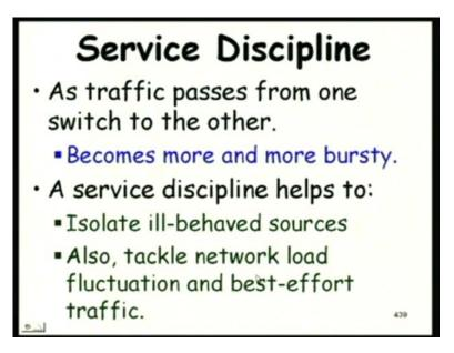
Or in other words, any traffic as it passes from one switch to other becomes more and more bursty. So, traffic that was bursty only to a small extent, will increase its burst size; and finally, after few switches it will become really bursty; the burst size would have increased ten times.
