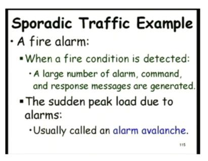
One example of a sporadic traffic is a fire alarm where very rarely a fire condition is detected, but once it is detected large number of alarm commands are sent out. There are response messages from these and may be action to be taken by sprinkler and so on. So,
