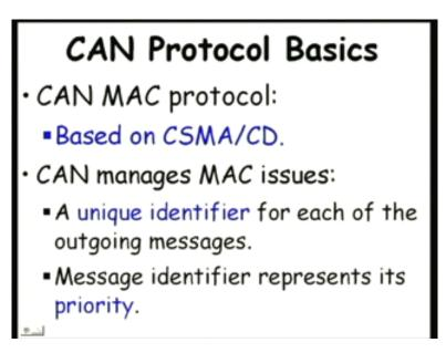
And the MAC protocol is that makes sense MAC protocol the Medium Access Control protocol is the CSMA/CD .CSMA/CD you know from a first course in networking. One implementation of the CSMA/CD is the Ethernet is very popular in traditional networking. CAN MAC is also CSMA/CD and here when CSMA/CD is used how does how do you assign priorities to different sources .Because you know there are some components whose messages need to be transmitted without delay.
