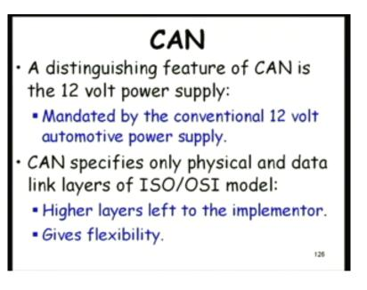
Another requirement was for it to operate at twelve volt power supply ,because all automotive vehicles operate at twelve volt supply and one thing that is important here is that it only its specifies the physical and data link layer and leaves the higher layers to the implementor gives flexibility.
