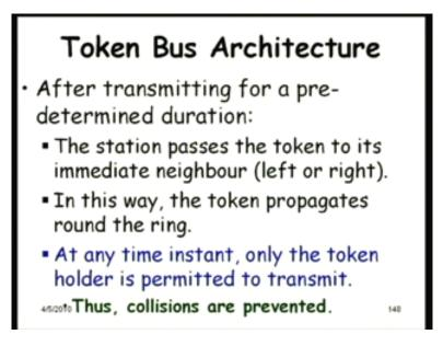
After transmitting its duration assign duration it needs to pass the token to the neighbor and a token propagates around the ring and. At any instant only one token only there is one token holder who can transmit. (Refer Slide Time: 52:11)
