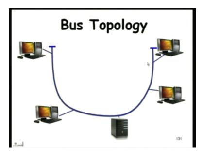
So let us check this out some properties of this. The bus topology as we know from a traditional networking course first level networking course is that there is a bus typically a coax cable and .Various types of computers attached to the bus and then it is the bus is terminated the terminators here in a coax cable.
