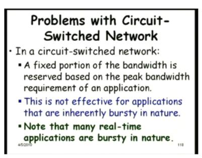
Let us see the problems with circuit switched network a fixed portion of bandwidth is reserved based on the peak demand and if the bandwidth requirement is constant then circuit switched network is All right, but that is rarely the case very rarely you will find that no the data is entirely constant. (Refer Slide Time: 12:53)
