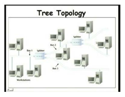
The tree topology is also popular when you have splitters and the different busses get arranged in the form of a tree.
