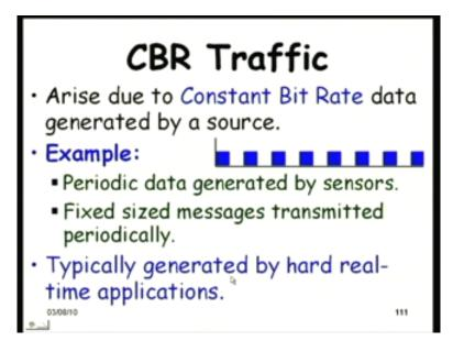
The constant bit rate data is generated by several types of sensors and also the commands to the actuators they are also in terms of constant bit rate. Overtime you see constant size data is being transmitted on the network.
