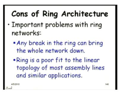
One major problem reliability issue. The other difficulty in using the ring architecture in real-time embedded application is that is a poor fit to the linear topology in most of the assembly line and similar applications.
