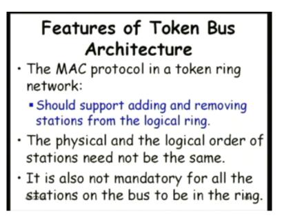
So, arbitration mechanism is simple collisions are prevented and of course, we should have protocols per how to add and remove stations in a token bus architecture or in the logical ring. Because they are may be stations which are part of the ring sometime and they might get excluded in some other time. The other thing is that the physical and logical order of the stations may not be the same and also all the stations on the bus need not be under ring. Is just an.(())
