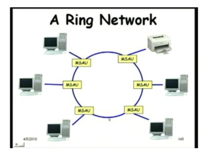
Look like this computers connected on a ring through which can be hubs where several problems with the ring architecture .One is that any break in the ring can bring the whole network down.
