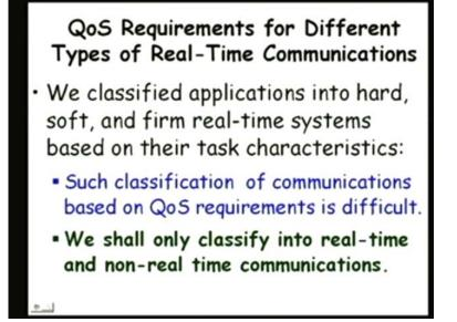
Now, let us see just examples of the quality of service requirement for different types of real time communications. Actually, if we remember that, when we discussed about the task characteristics of a real time system, we could classify them into hard real time task, a soft real time task or firm real time task, based on certain task characteristics.
