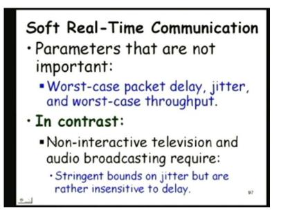
But there are some parameters which are not important, for example, the worst case packet delay, we do not really, it does not really matter if certain packets got delayed, as long as the average throughput is met, we do not bother, if some packets got delayed or they came very fast, we do not bother, jitter we do not bother.
