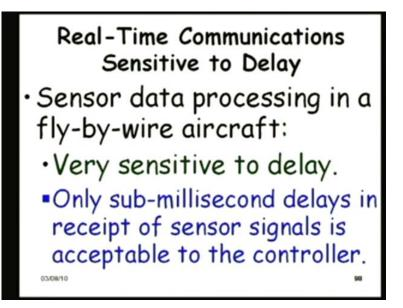
But let us look at another application, which is a sensor data processing in a fly by wire aircraft. So, an aircraft which is automated and there are no pilots in this, say fly by wire, so only ground commands can be given.
