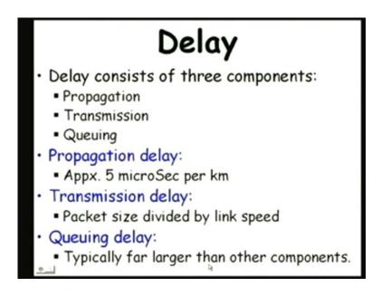
So, have you thought about this, that if you make a request for a web page clicked on the URL, which one, which of these components would be the one that is, dominating, I mean, where the maximum delay would occur? Queuing, it is the queuing delay, which is typically the largest delay in an internet situation, because the propagation delay is approximately 5 micro second per kilometer. So, even if it is 1000 kilometer you are
