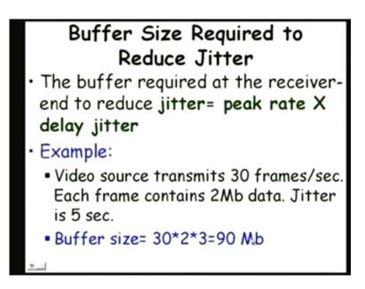
So, as the, we are not saying that the buffer size would eliminate jitter, we are not saying that, we are saying that it will smoothen out the traffic or the application that is using the data, will not feel as bad as when they are not buffered. So, it will reduce the impact of the jitter. Now, the idea is that, as the packet keeps on arriving, it keeps them in the buffer and if some packets are delayed, it can consume the packets that are there in the buffer.
