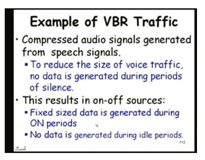
So, an example of a data of this type is the compressed audio signals generated from speech signals. Normally, when the voice traffic is sent on a network, you do not send any data during the periods of silence and possibly that is one of the reasons, why a transmission on a packet switch network is more efficient, then when you do transmit data on a connection based network.
