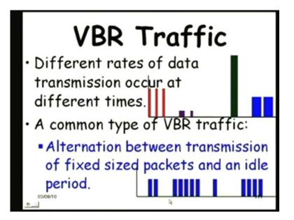
The variable bit rate traffic; here different rates of data transmission occur at different times. Let me not say transmission, we can say that data generation at the source transmission as different meaning. So, here the data generated by the source at certain time is let us say some 10 kilobyte of data generated per millisecond here, but at certain other time, it is 100 megabyte of data or something generated per millisecond.
