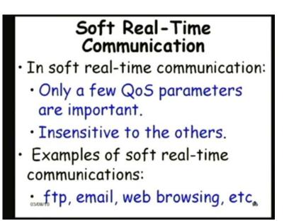
So, a soft or a non-real time communication is one, where certain quality of service parameters are important; it is not that, a non-real time or soft real time communication has no requirement on the quality of service, they have certain requirements.
