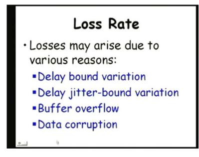
The transmission delay is only a very small part and loss rate is also another quality of service parameter; now, let us try to analyze, why losses occur in the network, what do you think, why losses occur in a network? The losses occur in a network, in a real time situation, due to many reasons, may be due to delay bound variation; the packet arrive too late to be used by the application, as far as the application is concern, the packet has been lost is of, no, use delay jitter-bound variation.
