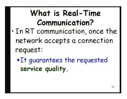
And in a real time communication, once the network accepts the connection request with specific demands regarding the parameters of the connection, it should guarantee the requested quality, requested service quality should be guaranteed by the network that is
