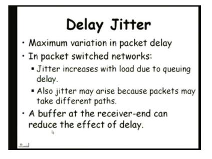
The delay jitter is defined as the maximum variation in the packet delay. So, each packet take certain time to reach, some packet arrive in let us say 10 millisecond, some packet arrive in 11 millisecond and some packet arrive in, let us say 9 millisecond and some packet arrive in 20 millisecond, not 20, let me just say 15 millisecond. So, what will be the jitter, they distributed around 10, let us say some are arriving at 9.
