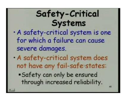
So, just to summarize what we discussed, a safety-critical system is one, where any failure can cause severe damage and no fail-safe sate exists in the safety-critical systems. So, cannot even revert to a fail-safe state.
