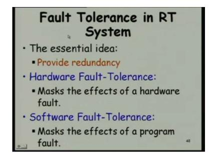
Fault-tolerance in hardware is very intuitive; if you talk to persons working in the hardware area, they say that yes, the hardware that we develop are fault tolerant and there are standard technique called as triple modular redundancy built in self test.
