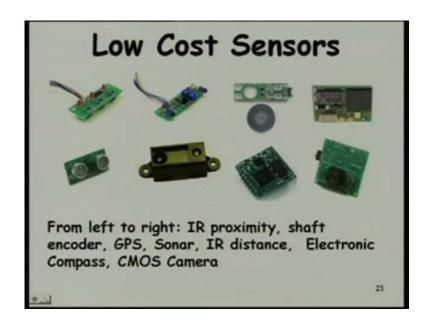
We can have, we know commercially have several low cost sensors that are available, the IR proximity server, the IR proximity sensor, the shaft encoder, GPS, SONAR infrared distance sensor, electronic compass, cmos camera, see the camera mounted here. So, these are various types of sensor you can buy of the self from shops and these are used to build the embedded systems.
