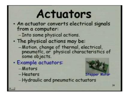
These are some of the actuators which convert electrical signals from the computer into actions, the actions can be in the form of a motion, changing the thermal characteristics or electrical characteristics, pressure, physical characteristics, so on.
