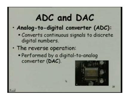
And off course most of these devices they use analog to digital and digital to analog converter, because most of the sensors they generate analog signals, where as our computer needs digital signals and similar is the case with respect to actuator. Most of the actuators they need analog signal, so a digital to analog converter needs to be done. Again these are available of the self; see here a small chip here is doing analogs to digital and digital to analog.
