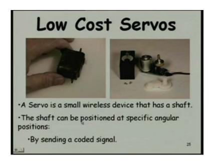
So, this is low cost servo used in many applications including the robos, it is a small wireless device that has a shaft and this can be positioned at specific angular positions by sending a coded signal very popular in robos.
