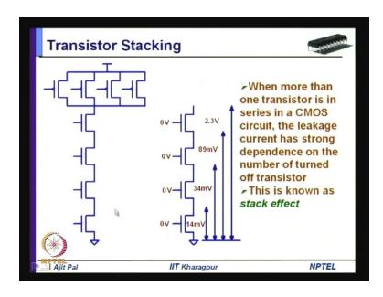
Coming to transistor stacking, whenever you are realizing circuit in this manner, say this is a four input NAND gate, so where you have got four n MOS transistors in series, and four p MOS transistors in parallel. Now whenever you do the stacking in this manner, there is a possibility some of the inputs will be 0, and some of them will be one; that means, you have got four inputs. So, there are 16 possible input combinations starting
