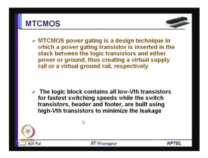
So, the logic block contains all low V t transistors for fastest switching speed, while the switch transistors; that means those sleep transistors header and footer, are built using high V t transistors to minimize leakage. So, basic idea here is you are not really sacrificing the speed of operation, because when the circuit is in normal mode, the sleep transistors are on.
