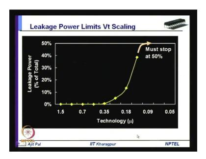
And I have already shown you this particular diagram; you can see the leakage power is increasing as you are going from one technology generation to the next technology generation. And requirement is that as it is crossing 50 percent of the total power, you must stop, somehow the increase in leakage power has to be stopped somehow, and what is that somehow, we shall discuss starting from today's lecture.
