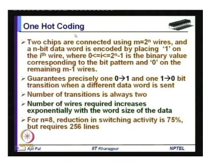
So, in this particular case what you are doing, say you have got one particular device maybe sender, then you are doing encoding and here you have got decoder and you have got your receiver, so this is you can say this is your receiver. In this case the n bit code that is coming from the sender is converted into 2 to the power n minus 1 bits on after the decoding; that means, decoder is converting to 0 1 1 in this way finally, it is 2 to the power n minus 1.
