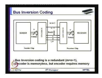
So, this is the example this is how it is being implemented you have the sender, and you have the encoder here which converts the n bit data into n plus one bit including this polarity bit. So, including this polarity bit the number of bits is n plus one so there is redundancy but redundancy is not much only one additional bit is added for transition over the Bus and decoder will convert it to n bit.
