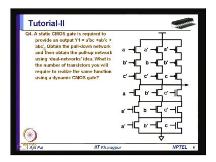
4th question static c mos gate is required to provide an output y one is equal to a bar b c plus a b bar c plus a b c bar. So, as we know.
