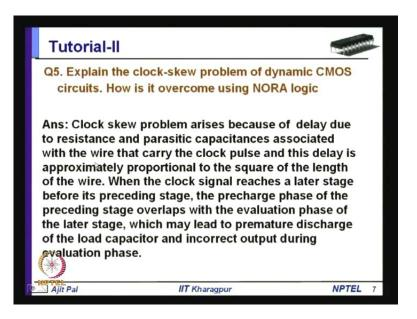
Coming to question number 5 explain the clock-skew problem of dynamic c mos circuit how is it overcome using nora logic as you know clock skew problem arises, because of delay due to the resistance in parasitic capacitance associated with the wire that carry the clock pulse and this delay is approximately proportional to the square of the length of the wire.
