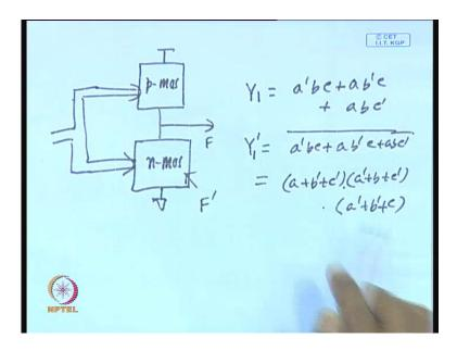
Whenever you are realizing a c mos circuit c mos gate you have got p mos network as pull-up device and you have got n mos n mos network as pull-down device and inputs are applied to both same inputs are applied same inputs are applied and you take the output from here and the n mos network is connected to ground cause it acts as a pull-down network this how realize the function.
