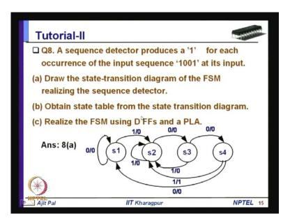
Coming to question number eight a sequence detector produces a one for each occurrence of the input sequence one zero zero one at its input draw the state transition diagram of the f s m realizing the sequence detector and obtain second part is obtained from the state transition diagram and third is realize the f s m using the d flip flop and p l a.
