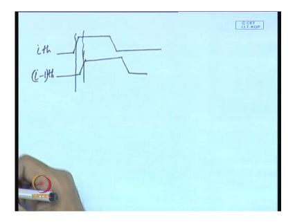
We have already seen discussed about it; that means, suppose this is the clock of one particular stage and this is the clock which has reached a I mean this is the clock of the preceding and succeeding stage and this is the clock of the succeeding stage; that means, this clock has reached the I x stage earlier than i minus one x stage.
