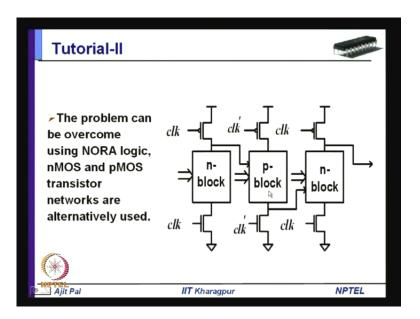
So, this problem as you know can be solved by using Nora logi,c where you are feeding the output of a of a dynamic circuit realized by n mos transistors, so n-block so output is going to a p-block.
