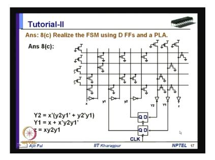
So, this is z x y two y one y one is equal to x plus x x bar y two y one bar and y two is equal to x bar y two y one bar plus y two bar y one as i have shown from this table.
