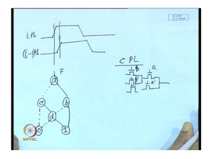
Which we have got let say a then dotted line is coming to c solid line is going to b and you have got a d and solid line from c is coming here dotted line from b is coming here and then you have got 0 dotted line from c will go to 0 dotted line from d is also going to 0 and then you have got one and the solid line from b will come to one and solid line from d will come to one this is the r o b d d that we get now from this you can very easily realize the past (()) network.
