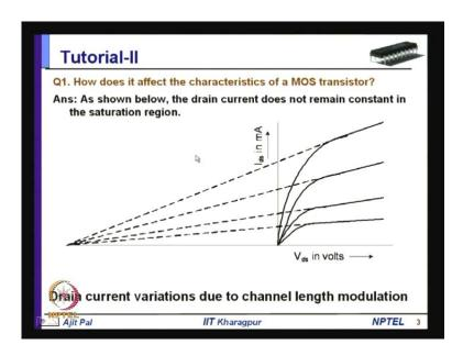
Shown in this diagram the variation of drain of drain current due to channel length modulation now.
