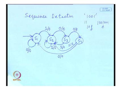
Sequence detector and that has to detect the sequence one zero zero one; that means, for each occurrence of one zero. One it will produce one now how do you dram the state transition diagram we have to consider an initial state let us assume this is the initial state s one initial state.
