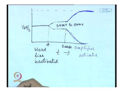
We can draw the circuit. So, initially there will be pre-charge both the lines will be precharged to v d d by 2 both the bit lines.
