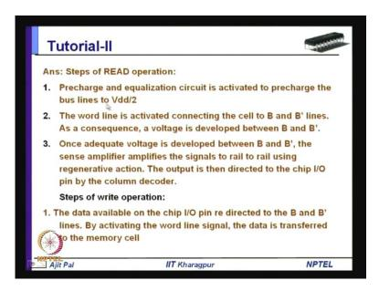
First you have to do pre-charge and equalization circuit is activated to pre-charge the bus lines to v d d by 2. So, there is a pre-charge and evaluation circuits which will be activated to make the bus lines zero.
