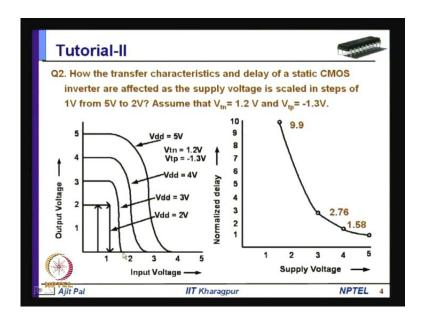
Coming to the second question how they transfer characteristics and delay of a statics c mos inverter are affected as you supply volt is scaled in steps of one volt from 5 volt to 2 volt assuming that V t n is equal to 1.2 volt and V t p is equal to minus 1.3 volt
