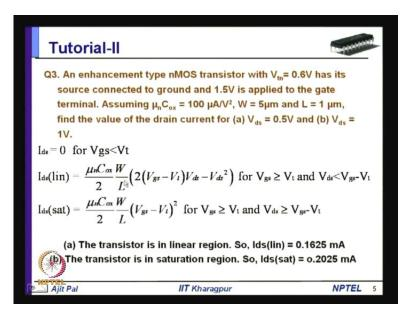
An enhancement type n mos transistor with v t n is equal to point six volt has its source connected to ground and one point 5 volt is applied to the gate assuming that mu n c o x is equal to hundred micro ampere per volt square w is equal to 5 micron and n is equal to one micron find the value of drain current for v d s is equal to point 5 volt and v d s is equal to one volt.
