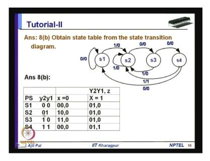
Now, you can very easily obtain the obtain the state table from the state transition diagram. So, you have got four states s one s two s three and s four. So, zero zero zero one one zero one one. That is the coding you have done the state assignment this step is known as state assignment it is not necessary that you have to use this code you could have used a zero zero zero one one one one zero you could have given that also.
