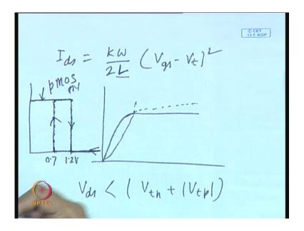
We know that when the when the v d s is less than v t n plus v t p then we get a kind of hysteresis.
