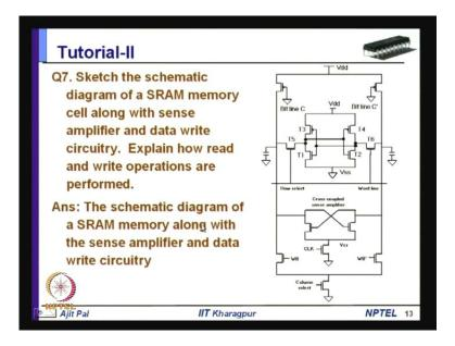
Now, coming to question number seven sketch the schematic diagram of the s ram memory cell along with sense amplifier and data write circuitry and explain how read and write operations are performed. So, this is the schematic diagram of a s ram memory cell. So, you have to explain the read and write circuits and you can see you have got a memory cell then you have got row select line and word select line row or word select line and column select line is here.
