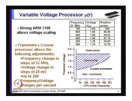
Now, coming to the first requirement, that is variable voltage processor. There are processors available, one is your strong ARM 11 00. This allows voltage scaling as you can see it can operate over a voltage range 1.1 to 1.65 and accordingly it can operate at different frequency that means when the supply voltage is 1.65 volt the operating frequency is 700 megahertz and this is the relative power 100.
