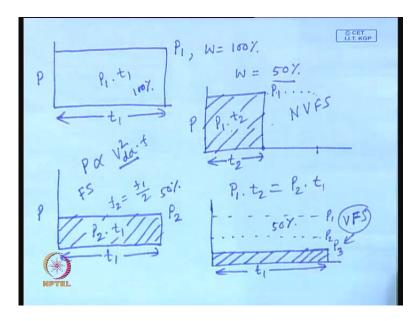
Here energy is significantly reduced and as you can see this is voltage and Frequency Scaling. This is only Frequency Scaling and in this particular cases neither no voltage nor Frequency Scaling and here also no voltage and Frequency Scaling, but here the workload is 100 percent, here the workload is 50 percent, here the workload is 50 percent and here also the workload is 50 percent. So, this is based on this. Now we shall develop
