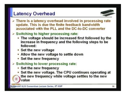
Another important parameter is latency overhead. As I have already told there is a latency overhead involved in processing rate update. This is due to finite feedback bandwidth associated with the Phase Lock Loop and the DC to DC converter, because this Phase Lock Loop and DC to DC converter these are analogue systems.
