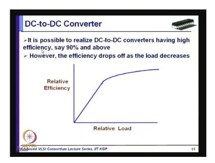
Now, coming to one very important aspect of DC to DC converter, as I have mentioned, it is possible to realize DC to DC converters having high efficiently say 90 percent and above. Unfortunately the efficiency drops off as load decreases; that means, when the
