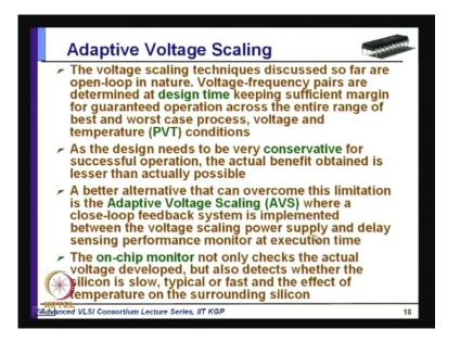
Now, the voltage scaling techniques discussed so far are open-loop in nature. Voltagefrequency pairs are determined at design time keeping sufficient margin for guaranteed operation across the entire range of best and worst process, voltage and temperature conditions that means you know those voltage frequency pairs are decided at designed time, although they keep on their applied at run time, but they are decided at design time.
