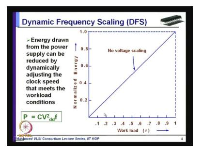
First we shall consider a simpler situation where the frequency scaled down as the workload reduces. So, in this particular case, as you can see, you were reducing the frequency as the workload is reduced. So, there is a linear relationship between the energy and the workload; so we can show you with the help of another plot. Let us
