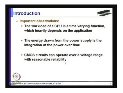
And these are the important observations; in fact the genesis of this Dynamic Voltage and Frequency Scaling will come from these observations. Number 1 is the workload of a CPU is a time varying function, which heavily depends on the application. For example, if you consider the workload of a CPU, we will find that with time it varies that means, it may somewhat like this; that means it is a time varying function and not only that, it will also depend on the class of the system.
