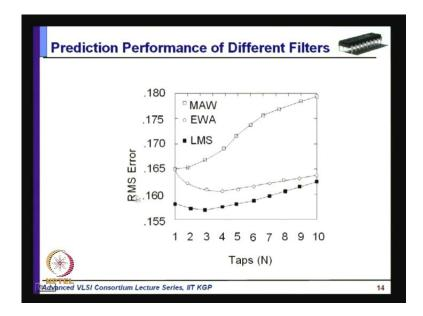
And this is the prediction performance of different filters is shown here. As you can see the RMS error root means square error is minimum for this LMS approach, this 1 m s approach. I have showed means least means square approach, where the error is minimum, error is maximum for this moving average window and this exponential weighted averaging gives you lesser than moving average window, but this LMS definitely gives you much less error compare to the other two schemes.
