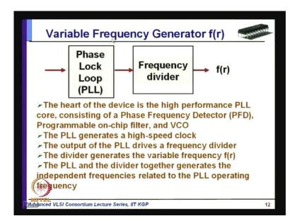
Coming to another important component, that is your Variable Frequency Generator. Variable Frequency Generator can be generated with the help of Phase Lock Loop. This is the traditional approach for generating variable frequency as you can see here there is a phase lock loop and the heart of this device is the high performance phase lock loop core consisting of a Phase Frequency Detector PFD and Programmable on-chip filter and a VCO, this is part of this Phase Lock Loop.
