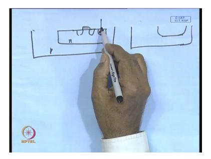
So, whenever you are realizing transistors of different voltages. As you know suppose, this is a n-well, this is a well this is a structure, and if there is a m o s transistor here, and this well is connected say suppose this is your n type and this is p type, and this is n plus this has to be connected to different voltages.
