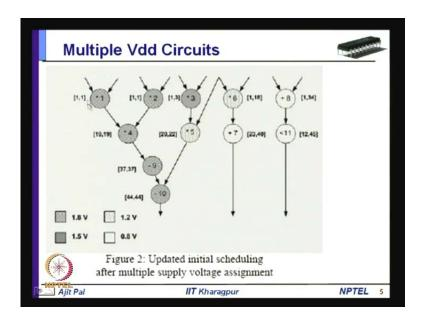
For example, in this particular case, we have the choice of 4 different voltage levels 1.8, 1.5, 1.2 and 0.84, 4 different voltage levels. As you can see the multipliers and adders which are on the critical path they have been given the voltage 1.8; that means, these modules will operate at 1.5 1.8. On the other hand, this multiplier is operating at 1.5 volt;
