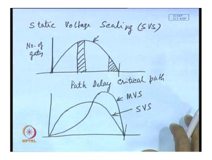
Say, we have already discussed about it static voltage scaling that is SVS. There if you consider different paths a circuit may have large number of paths, and if you plot the path delays this is the delay path delay, and on the y-axis it represents the number of gates on different paths. So you can see in this part you have got gates which are on very close to the critical path, because this is the critical path delay. On the other hand,
