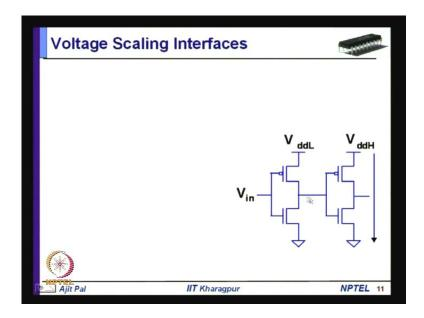
First, let us consider the voltage scaling interfaces. In this particular case, we have shown an inverter, which is in the lower voltage domain with supply voltage V ddL, and the signal is going from V ddL to V ddH. So, what kind of problem you will face in such a situation? (Refer Slide Time: 30:29)
