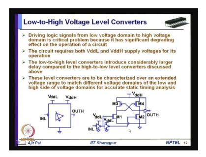
So, this I have already explained so you require a level converter to avoid this static power dissipation on this circuit, how can you realize a level converter? So, this is the type of level converter you can use.
