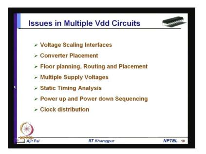
Now, we shall focus in various issues in multiple V dd circuits, we have seen how you can assign multiple voltages at macro level at standard cell level. It has got many challenges; that means, a circuit designer, if he wants to use multiple voltage domains or multi V dd circuits they have to face a number of challenges and they have to overcome them, what are the different challenges let us consider.
