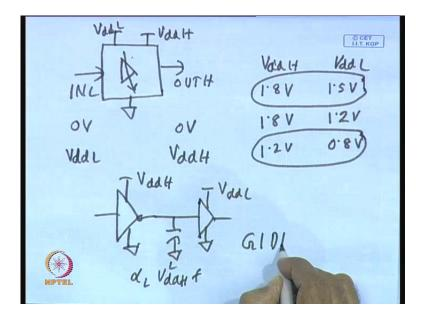
That means, you will require a level converter which is given the symbol there is a block it is receiving input at low level it is producing output at high level, and it is provided with V ddL to different voltage supply voltages V ddH and of course, there is a common ground. So, this is the symbol of a level converter in inside a symbol is given here which is essentially; that means, it is changing the level that it signifies that, and it can be realized by using a circuit like this.
