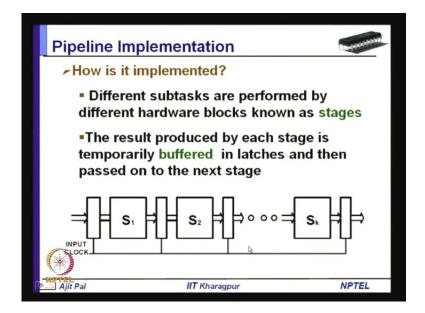
Let us see different subtasks are performed by different hardware blocks known as stages. So, a stage s one is performing subtask one s. That is performing subtask that in this way stage k is performing subtask k and you can see you are applying clock and you have got latches in between where intermediate results are stored and the clock transfers. The results from stage to other in a synchronous manner so this is how it is implemented and the execution is done in this manner.
