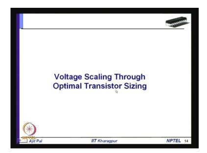
Now, we change here. And shift to another topic voltage scaling through optimal transistor sizing (refer time: 25:00) what do you really mean by transistor sizing. We know that a transistor can be realized with different length and width. So, whenever we increase the width what happen the resistance, decreases that means, if the width of a transistor is increased the resistance reduces.
