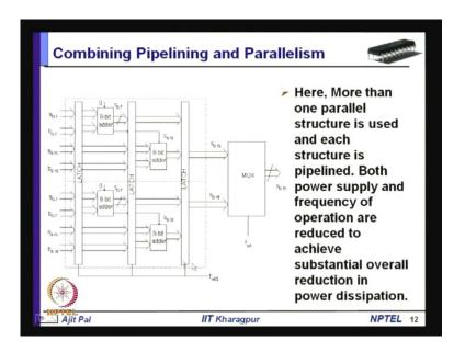
Now, we can combine pipelining with parallelism. So, earlier we have discussed parallel implementation today we have discussed pipeline implementation we can combine parallelism with pipelining that means we can have that parallel implementation and each of them is pipelined.
