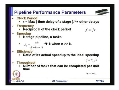
Now, in the context of pipelining, there are some performance parameter we use number one is clock period clock period. You know as we have seen when we go for implementation. We have to use some latches we have seen there and we have to apply clock. So, what is the clock frequency clock frequency is decided by the maximum time delay of the stage plus other delays due to latches and other things.
