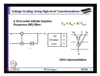
Now, let us focus on third technique voltage scaling using high level transformation whenever we are realizing some circuit can do high level transformation what kind of transformation. We shall do let me explain with the help of this example suppose, we have to realize a first order i i r filter infinite impulses response filter.
