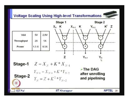
So, this particular stage can be pipelined how can it be pipelined you can see in the stage one we shall compute z some intermediate result then z will be used in the second stage to produce the y n minus one and y n. So, there the implementation will be somewhat like this say.
