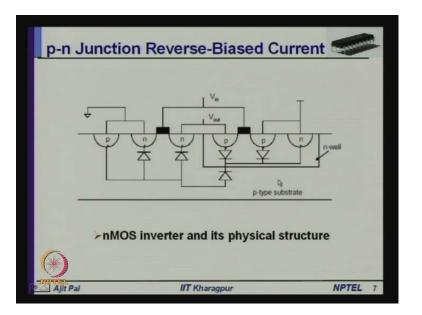
So, we can draw the diodes as you can see all the diodes are shown here, so this is the within the geometry of the device, there are some junction diodes, which are present; because, of the way the nMOS transistors are realized. And during normal mode of operation, these diodes are reversed biased, that is why it is called reversed biased leakage current.
