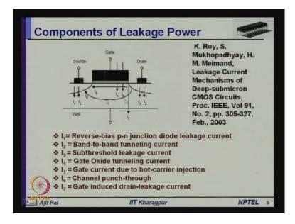
Now, we shall focus on leakage power dissipation and first, we shall discuss about the different components of leakage power. I have already told, that the leakage essentially can be divided into three types of leakage, gate leakage and that diode leakage, gate leakage and the leakage through the channel. So, there will be sub threshold leakage you can say, there will take different types of leakage currents.
