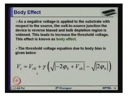
So, this is the, that is the reason why whenever reverse body bias is increased, threshold voltage is increased. On the other hand, you can apply a positive reverse voltage to substrate
