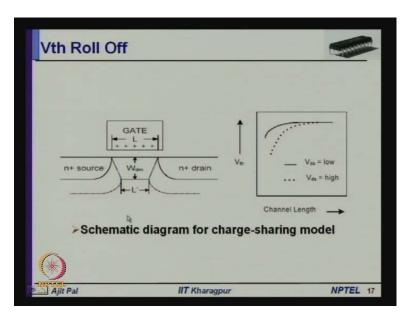
And let us consider the Vth Roll off you know normally, the gate voltage the your applying supply some voltage to the gate also, your applying voltage to the drain. As you know to attract the electrons from the source your, you apply positive voltage to the drain that is how the current flows.
