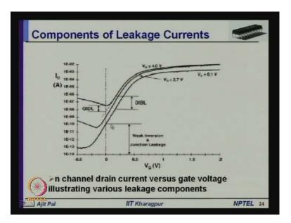
And in this particular diagram different types of leakage currents that, I have drawn explain are shown a summary of that is, shown here. For example, this is the 0 gate voltage, where there is a quadrant current, because of weak inversion, there is sub threshold leakage current and junction leakage current. And then, because of d i b l effect drain-induced barrier lowering and gate-induced drain leakage current you can see there are more currents I mean currents are increasing.
