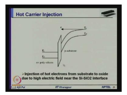
Now, there is another you know gate leakage that is known as hot carrier injection. You know, whenever you are applying a gate voltage. May be whatever may be very small, but because of the smaller thickness of the silicon dioxide layer that electric field is so, high that it creates some electrons of very heavy, very high energy. That means electrons acquire very high energy, those are known as hot electrons.
