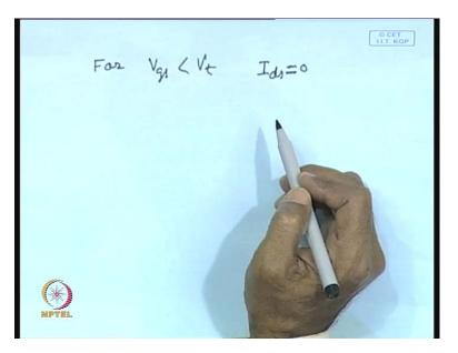
Normally, we know that, you know normally, we assume that for V g s less than V t, I d s is equal to 0 that means, there is no channel, if the gate voltage is less than the threshold voltage. And drain current will start flowing only when the gate voltage is larger than the threshold voltage of the device, but in practice that is not true. Particularly when the gate voltage is increased from 0 and it becomes closer to the threshold voltage.
