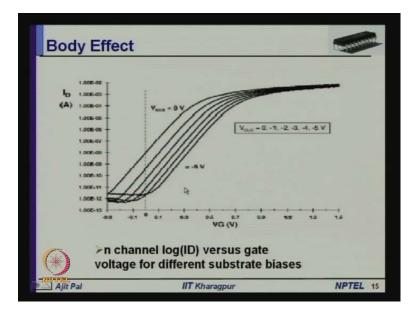
So, you can see in this particular curve, the how the body effect is changing the drain current so, here there is a plot of on the x-axis you have got the gate voltage, on the y-axis you have the drain current in logarithmic form. So, it is a kind of log linear curve, so y-axis log, logarithmic and x axis linear, that is gate voltage is linear now, you can see when the 0 gate voltage is there, even then there is a current flow.
