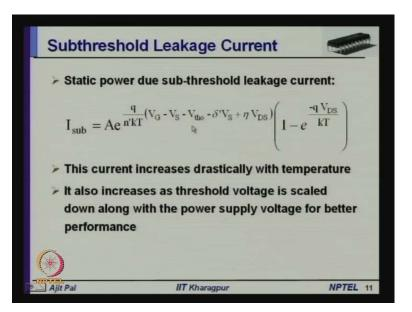
And here is the expression for the sub threshold leakage current, A is kind of constant primarily depends on the fabrication, length, width and various other parameters. Then, q be q by n das K T, V G is the gate voltage, V s is a substrate voltage and VT 0 is essentially the threshold voltage with 0 body bias, 0 bias of the, 0 bias on the substrate. And this delta das V s is the is due to the to take into account the body bias effect.
