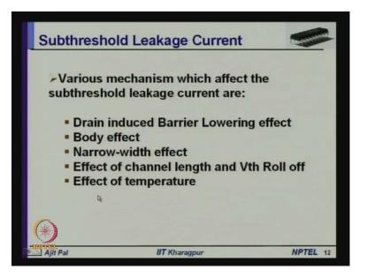
And this sub threshold leakage current has dependence on a number of parameters, there are various mechanism which contributes to the sub threshold leakage current. One is your I have already mentioned drain induced barrier lowering dibble effect, second is body effect, third is narrow-width effect, fourth is effect of channel length on and Vth Roll off and there is impact of temperature, effect of temperature.
