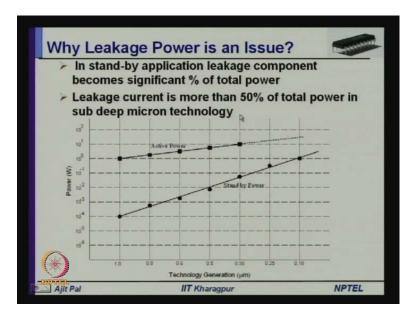
Now, let me conclude with another very important point, particularly the leakage current; you can then we I have to two lines the top one is drain current, the bottom one is leakage current or standby current. You can see the slope of this is larger than the other one that means, the leakage current is increasing at a faster rate, than, the than the active current active current or you can say dynamic current.
