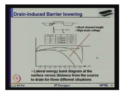
So, let us very briefly consider, how the threshold sub threshold leakage current is affected, because of these effects. First of all drain-induced barrier lowering, in this particular diagram, as you can see I have plotted the lateral energy band diagram, at the surface versus the distance. So, you can see here, this side is the source and this side is the drain so, here this is the y by L, length is a channel length.
