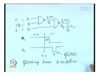
Let us consider a very simple circuit, we have two NAND gates let us assume, here is one NAND gate and this output is fate to another NAND gate to input NAND gate. Here, you are applying A and B as input and another inputs C is applied to the third gate. Now suppose, the initially the value of A, B and C is say 0 1 and 0, that is being applied and so how it will be the output at output 1 and output 2, since as you know in case of a NAND gate if any of the inputs is 0 output will be 1.
