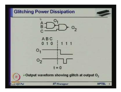
So, let us start with glitching power dissipation, earlier I have mentioned about the occurrence of glitch in CMOS circuits. As I mentioned, the glitch occurs in a CMOS circuit, because of finite delay of the gates, let me take up an example.
