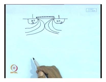
So, this is the mos transistor again I am drawing, say this is your say source n plus n plus Source, so this is Source this is drain. Now, whenever; and this is the gate region here, you have got poly-silicon layer, silicon on top of silicon dioxide. Now, whenever you apply a positive voltage there is a there is you know, this is the depletion region now, as you increase the drain voltage what happens these depletion regions widens.
