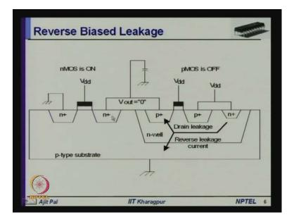
First let us focus on reverse biased leakage current, first from this reverse biased leakage current occurs, here we have got a CMOS inverter shown here. So, you can see this is the
