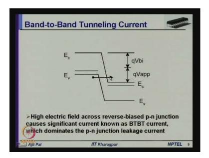
For example, there are two types of diode currents this is 1, another one is known as band-toband tunnelling current. In fact, in deep sub-micron technologies, this band-to-band tunnelling current is becoming higher than the reverse biased diode leakage current. What is band-to-band tunnelling current? You know those diodes we are, we have told those are reverse biased and because, of reverse biased diodes a voltage is developed across those diodes.
