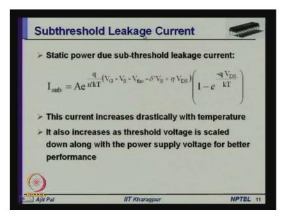
Now, let us focus on sub threshold leakage current. The sub threshold leakage current is a very significant, components of the leakage power and this current passes from drain to source through the channel.
