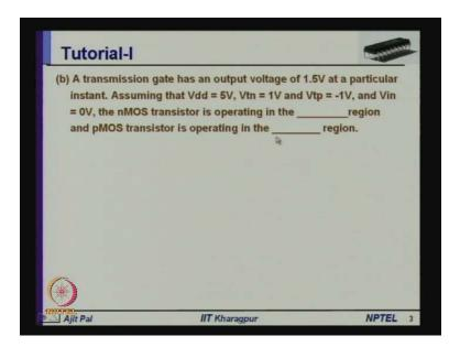
Second question was a transmission gate has an output voltage of 1.5 volt at a particular instant, assuming that V d d is equal to 5 volt V t n is equal to 1 volt V t p is equal to minus 1 volt and V in is equal to 0 volt. The n MOS transistor is operating in the dash region and p MOS transistor is operating in the dash region.
