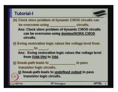
So, that is the job of the swing restoration logic, it raises the voltage level from V d d minus V t n 2 V d d. Next question is, sneak path leads to some problem in pass transistor logic circuits, what kind of problem it can lead. Again, in this case it leads to undefined output.
