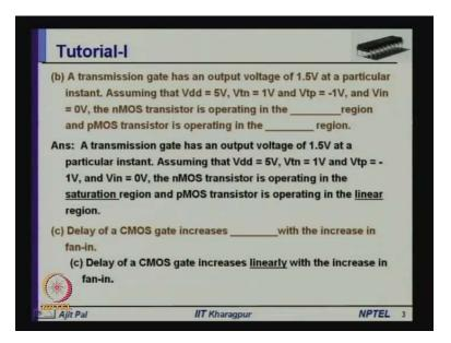
So, the answer is, the delay of a CMOS gate increases linearly with increase in fan-in. But the increase in delay that occurs in to two different ways, in two types of gates. In case of NAND gate it is, because of the delay of the series n MOS transistors. In case of nor gate it is, because of the delay of series p MOS transistors, that you have to keep in your mind.
