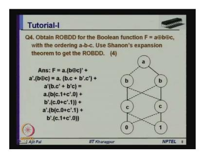
Coming to the last question, obtained ROBDD for the Boolean function F with the ordering a b c. Problem is, F is equal to a exclusive or b exclusive or c. Use shanon's expansion theorem to get the ROBDD. Here is the Shanon's expansion, and b expand it again.
