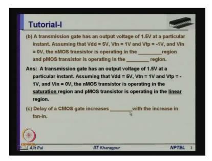
I have written it just the opposite by mistake, this here is a type of; that means, it will be in linear region n MOS and p MOS will be in saturation region. Now, coming to the third question; delay in CMOS gate increases with the increase in fan-in. So, how the delay of a CMOS gate increases, both for NOR and NAND.
