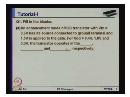
So, first question was, essentially a fill in the blanks question. It was an enhancement n MOS transistor with V t n is called 2.6 volt, has it source connected to ground terminal, and 1.5 volt is applied to gate. For V d d is equal to 0.4 volt 1.0 volt and 3 volt, the transistors operates in the dash dash and dash respectively. So, in what regions they really work, that has to be decided.
