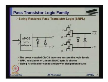
So, this is how you can realize different gates with the help of CPL technique. Now coming to the second family member, swing restored pass-transistor logic.
