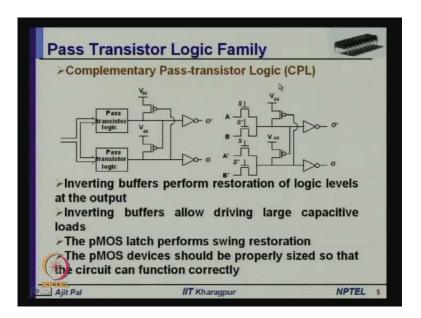
So, let me introduce the first family member; that is your complementary pass-transistor logic CPL. So, CPL or complementary pass-transistor logic, CPL as the as its name suggests complementary, complementary means it has got both the outputs, complementary outputs; that means, f and f bar; that means, it is dual-rail.
