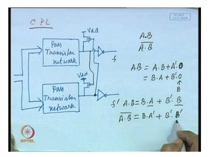
So, what is being done? Two networks are used; one is your one for realizing f; another for realizing f bar. So, it will have a one pass-transistor network and you will require two pass-transistor networks to realize the complementary function. So, another pass-
