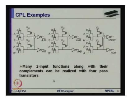
However proper sizing of this pass transistors is necessary, to avoid unnecessary power dissipation and delay. And using the same concept we can realize different types of gates by using this CPL technique, you can see here OR and NOR has been realized and in the same way, you can realize the pass-transistor network. And here, we have realized the XOR and XNOR again by realizing the p, the pass-transistor network using Shannon expansion theorem.
