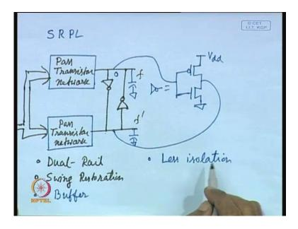
So, in swing restored pass-transistor logic so, this is SRPL, swing restored pass-transistor logic. In swing restored pass-transistor logic, what is done? Again two pass-transistor network is used like the previous case. So, you have pass-transistor network pass-transistor network and you will require two pass-transistor networks. It may be noted that the number of transistors required in each network will be same; only difference will be
