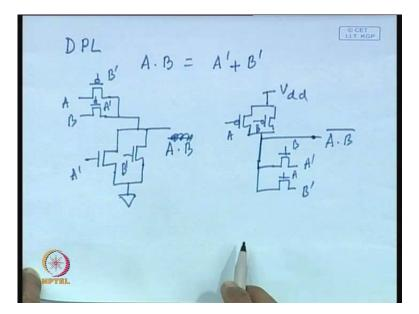
So, far as if pass-transistor is concerned, you were using only nMOS transistors. But in case of DPL, you will see both nMOS and pMOS transistors are used and typically the
