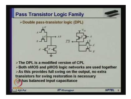
Coming to the third family member, which is known as double pass-transistor logic DPL; in case of DPL, again you are using dual pass-transistor logic DPL; you are using both nMOS and pMOS transistors earlier we have seen.
