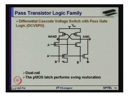
So, this is the fourth member of the logic family coming to the last member of the logic family which is differential cascade voltage switch with pass gate logic DCVSPG.
