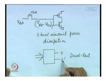
So, you have to use some swing restoration circuit to overcome multi-threshold voltage drop. As we know, whenever the signal passes through a pass single or multiple pass-transistors. Even if you apply V d d here; you will and the gate voltage is V d d, you will get V d d minus V t n.
