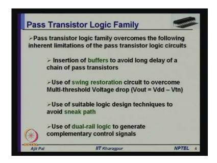
Now I shall introduce to you the pass-transistor logic family. Obviously, the passtransistor logic family has been, I mean has been provided, has been has been merged such that, it overcomes the various limitations of pass-transistor logic circuits. We know that there are a number of inherent limitations of pass-transistor logic; these inherent limitations are overcome with the help of these logic families and I shall introduce to you various members of this family.
