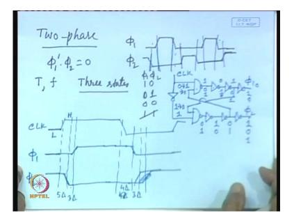
So; that means, you will be having a clock phi one another clock phi two. So, and they will have some this kind of relationship phi 1 this is phi 1 and phi 2 will be like this they are called non overlapping. By non overlapping we mean, they are never simultaneously
