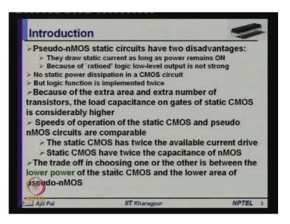
Coming to the introduction, we have seen that pseudo-nMOS static circuits have two disadvantages. So, they draw static current as long as power remains on and, because of ratioed logic, low-level output is not strong. On the other hand, there is no static power dissipation in CMOS circuits, but logic function is implemented twice.
