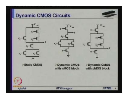
So, we can realize dynamic CMOS circuits by extending the idea of static CMOS and here, as you can see how we can do that. Whenever we are using uh statics I mean, by dynamic circuits by using CMOS instead of the nMOS transistor let me redraw it again.
