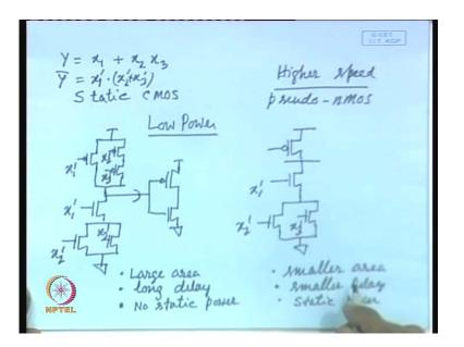
Let me consider a very simple function say you have to realize y is equal to  $x \ 1$  plus  $x \ 2$  x 3. So, using static CMOS, what will you do? You will realize this function you have to take compliment of this; that means, this will be the compliment of this is x bar dot x 2
