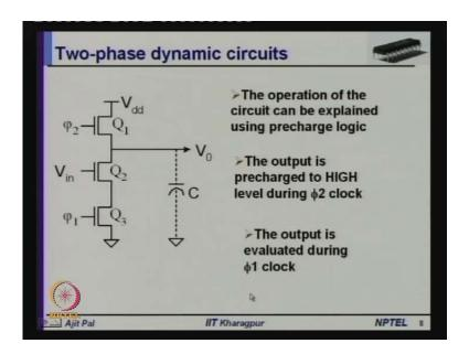
Now, let us see how we can use this two-phase clock to realize a two-phase dynamic circuit let us consider a two-phase dynamic nMOS inverter.
