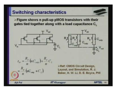
So, with this conclusion in mind let us now move to discuss about the switching characteristics. So, whenever we consider the switching characteristics, the figure shows n pull-up pMOS transistors with their gates tied together along with a load capacitance C l. So, for the sake sake of simplicity what we have assume, as if all the NOR gates are tied together pMOS transistors are tied together, that is the difficult NAND configuration and this is connected to C L.
