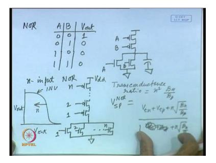
So, 0 0 0 1 1 0 and 1 1 and V out for NOR gate when it will be 1 it will be 1 for as you know for or gate the for these three output is 1. So, in this case this will be 0 and only for 0 0 outputs will be 1 that will be the case for NOR gate. So, how that can be realized? So, when both of them are 0 then output is 1 so that means, what you have to do we have
