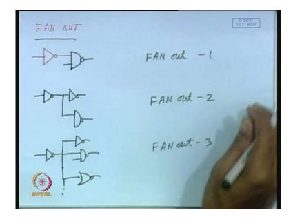
So, fan-out fan-out is essentially the number of gates the a particular gate is driving for example, this inverter may be driving several gate say it can drive only one gate it is going to one input of a NOR gate. So, in this case fan-out is equal to is one or it can drive more than one gate say, it is driving an inverter as well as it is driving one NAND gate. So, in this case the fan-out is equal to 2 similarly, it can drive a several gates for
