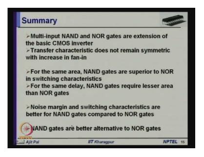
So, here is the summary of different types of whatever we have discussed today. So, multi-input NAND and NOR gates are extension of basics CMOS inverter we have discussed. How the how the multi-input NAND and NOR gates can be realized by extending the basic concept of an inverter, by adding more and more number of transistors as the fan-in increases. And we have seen the transfer characteristic does not
