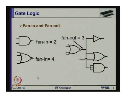
First let us focus on fan-in and fan-out. So, let us consider what is fan-in fan-in fan is essentially the number of number of inputs.
