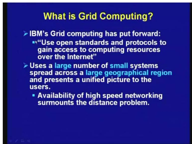
So, IBM's grid computing has put forward that actually basic idea was use open standards, and protocols to be an access to computing resources over the internet. So, you are gaining a access of computing resources over the internet, and you are using large number of small systems spread across a large geographical area region, and it presents unified picture to the users. So, here also it is giving some kind of unified
