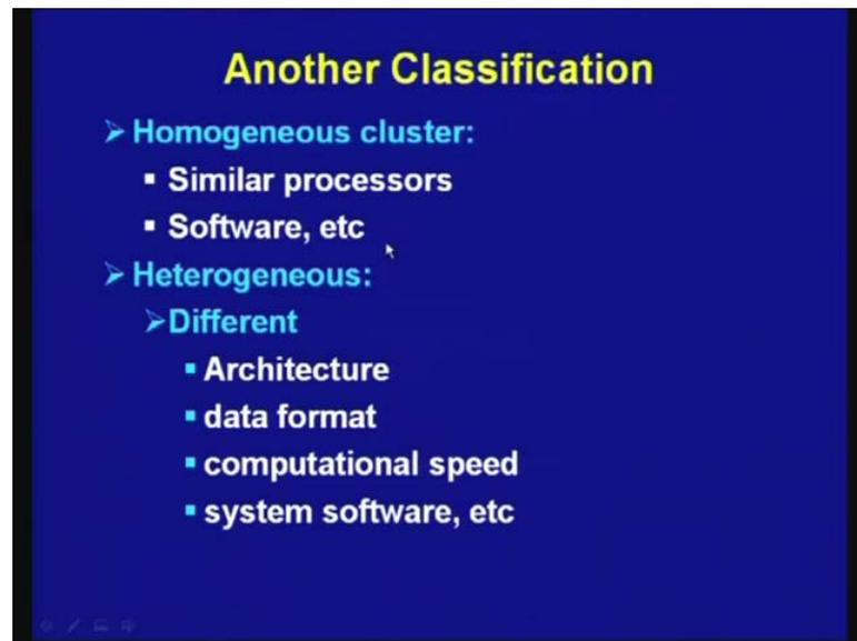
Then you have got, you can have homogenous cluster another way of classifying is homogenous and heterogeneous, so homogeneous cluster will have similar processors. So, all the nodes will be identical or similar software operating system, and software present in all the components, all the nodes in cluster. Alternatively you can have heterogeneous system with different architecture, data format, computational speed, system software that means, operating system and so on.
