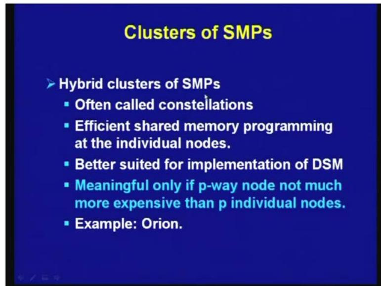
Then you can have cluster of shared memory multiprocessors, so highbred cluster of shared memory multiprocessor can be used, this is often called constellation. So, this is efficient shared memory programming at the individual node is possible, because each is having a shared memory multiprocessor. So, this is better suited for implementation of distributed shared memory multiprocessor, and this is meaningful only p-way node not much expensive than p individual nodes.
