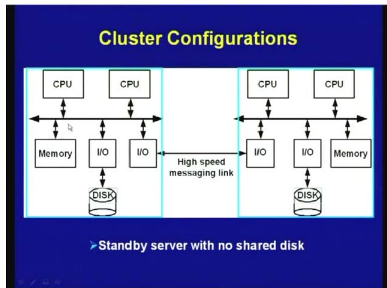
Here you have got two computers shown here, I mean here you have got one you can say, number of processors connected to a shared bus and this is connected to another system, which is also I mean multiple processor and which shared memory. So, these
