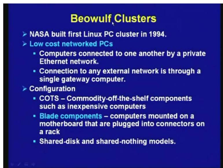
This is an example Beowulf cluster, NASA build first Linux PC cluster in 1994, so it is a low cost network PC's computers connected to one another by a private Ethernet network. So, connection to any external network is through a single gate way computer, and configuration is you are having commodity of self components, such as inexpensive computers. And blade components are use that means, the computers mounted on a mother board that are plugged into connectors on rack.
