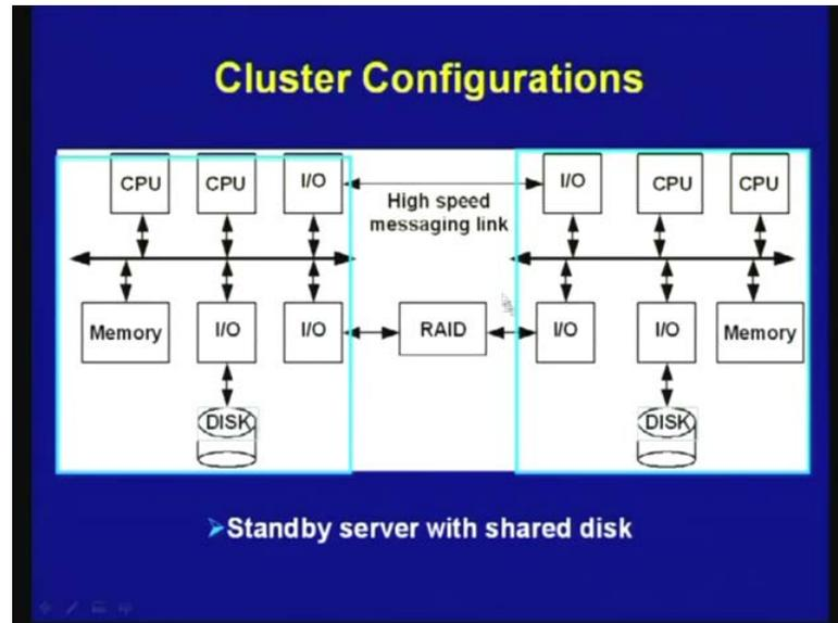
This is another configuration, in which you can have not only high speed messaging link, but you may have a shared hard disk, so in the form of redundant array of independent disks. So, here a raid is shared by these two systems through I O buses, so this is stand by server with shared disk.
