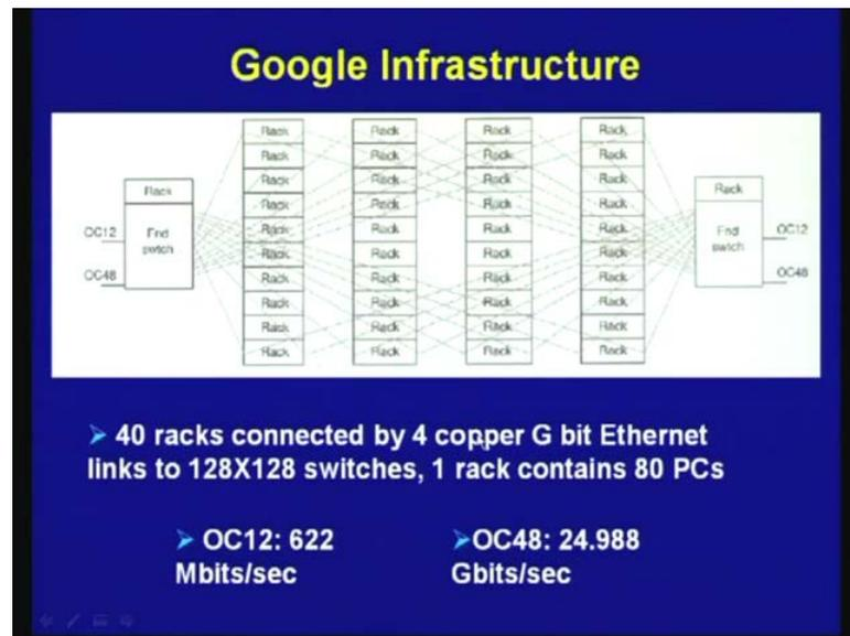
So, this diagram shows Google infrastructure, you can see here different rack shown 10 racks in here, 10 racks here, we have got 40 racks connected by 4 copper Gigabit. And that links 128 into 128 switches, so we have 128 into 128 switches and 1 rack contains 80 PC's. So, each rack is containing 80 PC's and you have got 40 such racks, so you can imagine the total number of such some PC's have represent here.
