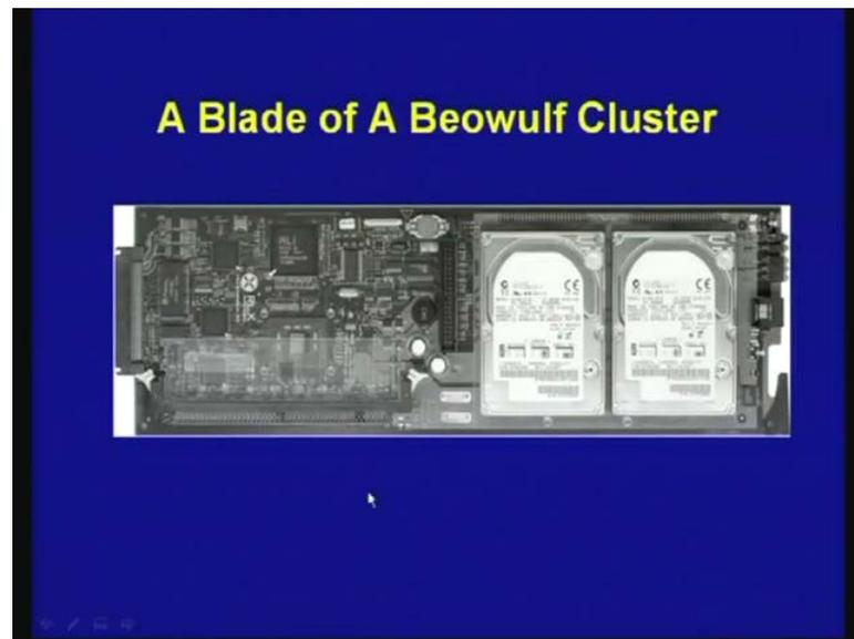
This shows a single Beowulf cluster, as you can see this is the connector which can be connected to the back plane. And here it shows two processor, this is one processor, this is another processor to two processing module, which are present in a single blade.
