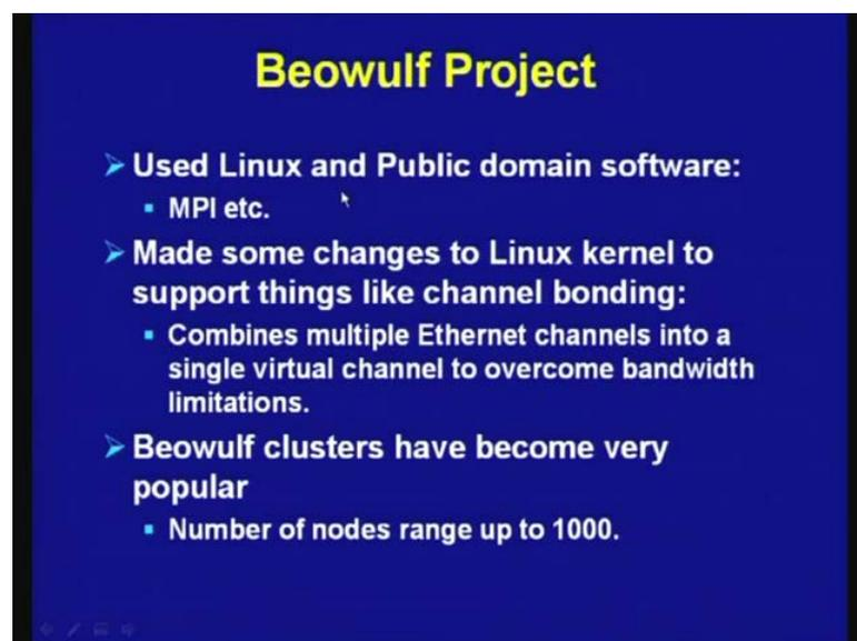
And this Beowulf project of NASA used Linux and public domain software, so they did not go for any custom software, so custom software is not being used, standard commodity of the software has been used. So, made some changes to Linux kernel to support things like channel bonding, so you have seen multiple Ethernet channels are
