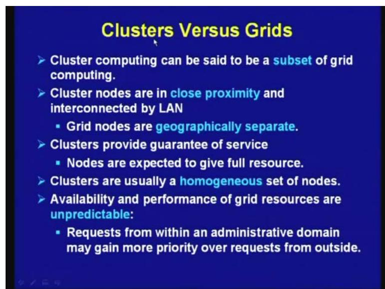
So, here is a comparison between cluster computing versus grid computing, so as I mentioned cluster computing can be said to have a sub set of grid computing. Because, cluster nodes are in close proximity, and interconnected by LAN as I have mentioned, and grid nodes are geographically separate and connected through wide area network or WAN. So, clusters provide guaranty of service, nodes are expected to the full resource on the other hand, clusters are usually heterogeneous site of clusters.
