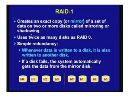
So, this is your RAID level 0, and a this was how it really works coming to RAID level 1, so this creates an exact copy of a set of data on 2 or more disks called mirroring or shadowing, so in this case what we are doing to improve the reliability and availability.
