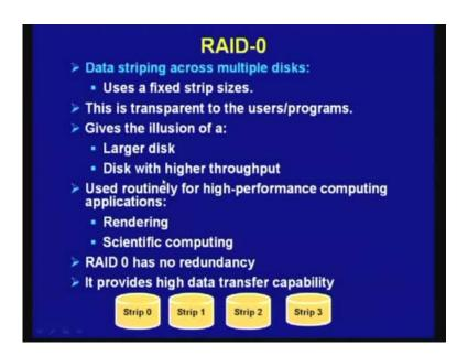
So, as I mentioned there are 6 different RAID levels, first one is known as RAID 0, so although you are using the terminology redundant, as we shall see in case of RAID level 0. There is no redundancy, and the main thing that is being done in RAID level 0 is data stripping across multiple disks, so uses a fixed strip sizes and this transparent to the users or programs, and what is being done.
