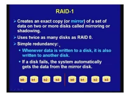
So, in this case this is the very simple redundancy and very simple, and that widely used in many applications in the early years of redundancy, and whenever data is written to a disk it is also written to another disk. So, in this particular case I mean reading can be done either from this disk where block 0 is stored or can be you can read it either from the disk.
