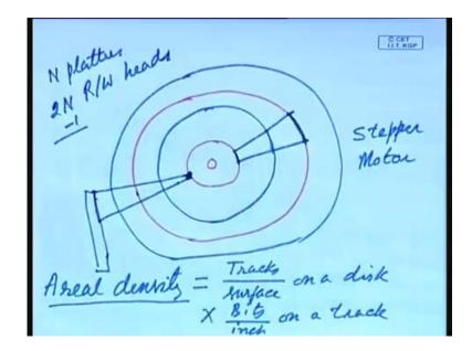
So; that means, what happens your read write head if this is read write head, if it is pointing to track number 0. So, it can move in this direction track sorry track number 0 is this 1, track 0, track 1 in this way it can move with the help of motor that is called stepper motor, with the help of a stepper motor the read write head is positioned on different tracks of a surface. And this read write head assembly, you can say all the heads on different surfaces move together.
