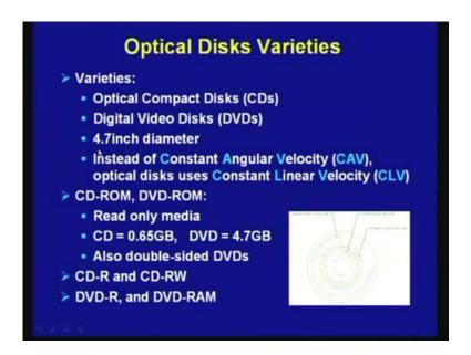
So, this gives you shows you different varieties optical compact disk, Digital Video Disks DVDs, 4.7 inch diameter. So, one new technique that is used here is instead of constant angular velocity, optical disk uses constant linear velocity.
