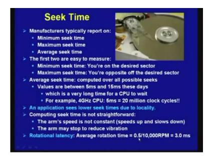
So, that is actually decided by the rotational latency, and average rotation time is roughly half of the worst case time that is your 0.5 by 10,000 RPM if this speed is 10,000 revolutions per minute. So, that is roughly equal to 3 millisecond, so you can see rotational latency is of the order of 3 millisecond.
