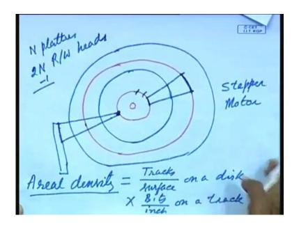
What is rotational latency, we have seen that seek time is the time required to position a read write head on a particular track, now you have to place it on a particular sector.
