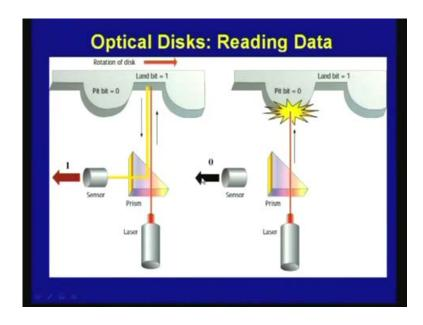
So, this is shown with the help of this diagram, so in this particular here as you can see, this is the light source, laser source. So, which is falling on the land, so which is
