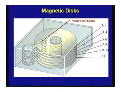
And this is a magnetic disk, as you can see you have read write heads, these are the read write heads. And each of them is representing a platter and as you can see, each plate is having 2 sides; that means, 1 and 2 corresponds to 2 sides of platter 1, 3 and 4 corresponds to 2 sides of platter 2, 5 and 6 corresponds to the 2 sides of platter 3 and so on. Of course, the last platter you cannot really access the bottom side that is why only 11 surface is shown 12'th surface is not accessible.
