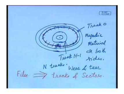
That means, in a, so far a programmer is concerned he is concerned about the files, he stored different files. And these files have to mapped to different tracks and different sectors of a track that mapping is done that information is stored in this File Allocation Tables or FAT.
