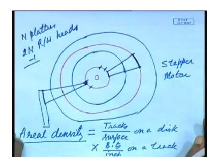
So, earlier we have seen that angular velocity is small because, you know the, so when the read write head is here, the time that is required to read for this part is same as the this part, so angular velocity is same.
