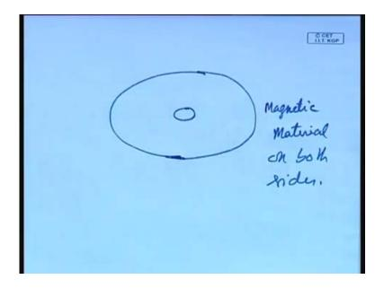
So, you can say this is a platter circular disk and a magnetic material is deposited on both sides.
