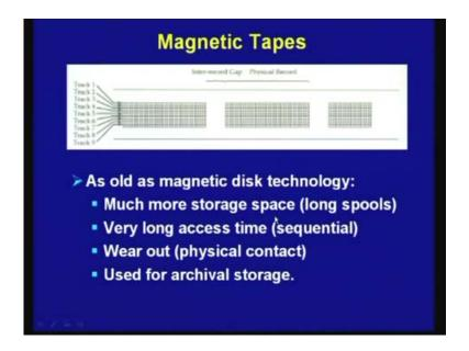
Then comes the magnetic tapes, this is as old as the magnetic disk technology, much more it has got much more storage space, very long access time. So, you can see here on a it is in the form of a tape just like your audio tapes, so on a single tape it is having a number of tracks, track 1, track 2, track 3, track 9. So, you can transfer parallelly, a number of bits different bits, so 9 bits you can transfer parallelly, whenever you are you are reading from a tape.
