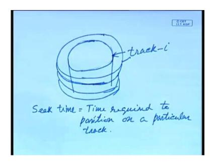
Suppose this is one platter, then at the bottom of this there is another platter, then there is another platter, then there is another platter in this way you got large number of platter. Now, let us consider the read write is positioned to track number i, so track number of i of this platter on both surfaces, than the track number i of the other platter on the same
