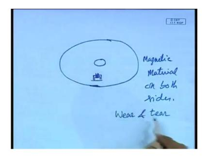
So, there will be wear and tear because, that magnetic surface is coming in close contact here for example, this is the electromagnet. So, it will come in physical contact as you can sequence with the magnetic material will get I mean eroded with time that is the reason why, the life of a magnetic disk is not very long.
