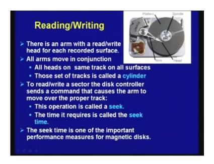
Now, how you are performing reading and writing, so there is an arm with a read/write head for each recorded surface. So, there is separate read write head you can see this is one here, separated read write head, which is available for each surface, so all heads on this same track on all surfaces, so what happens that all the heads move together.
