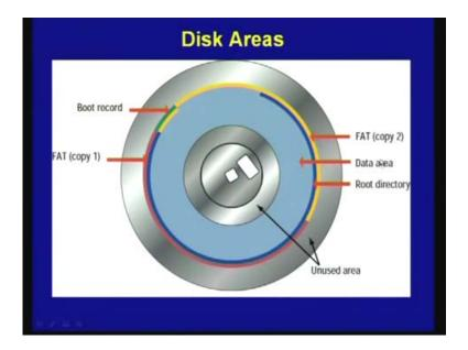
As you can see in this diagram different areas are shown, so that boot sector is that green portion is the boot sector, then is that File Allocation Table FAT that read track. And that file allocation table is duplicated for the purpose of I mean higher redundancy, so there are two file allocation tables stored as you can see two FAT, FAT copy 1, FAT copy 2. Then root directory that blue circle blue track is showing the, so you have started in this way first the boot sector, then the FAT.
