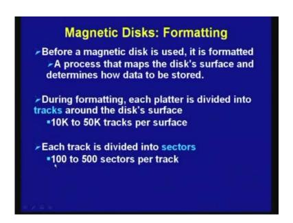
And the number of tracks is increasing with advancement of technology as you can see, it can vary from 10 K to 50 K tracks per surface, on a single surface you can have 10,000
