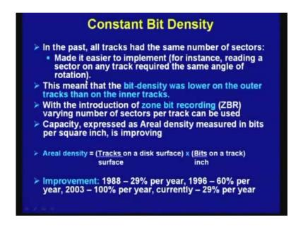
Now, in the past all tracks had the same number of sectors, as I have already mentioned, and this made it easier to implement, implement means for instance reading a sector on a track required the some angle of allocation rotation.
