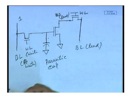
And then you are taking the output, with the help of again 2 transistors. This is your, this is your, this is connected to that word line and this is connected to bit line and this is also connected to bit line. So, this is bit line read and this is bit line write. So in this case, the operation is different. Here you are applying write line write signal and for read you are using, this is for write, this is for, this is for write and this is for read.
