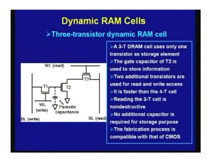
So in this 3 transistor cell, here you are not using 4 transistor, but you have a single transistor and the get capacitance of this transistor is used to store information.
