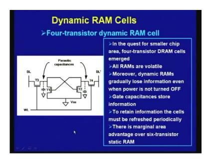
As I mention, the number of transistor in static RAM is quite large – 6. So, if you want to reduce the number of transistors, then we have to go for some other techniques and that has lead to dynamic RAM cells. So it started with and 4 transistor dynamic RAM cell, as we shall see, this dynamic RAM technology has involved over the years, so starting with 4 transistor cell to single transistor cell. For example, in this particular diagram, you have got 4 transistors.
