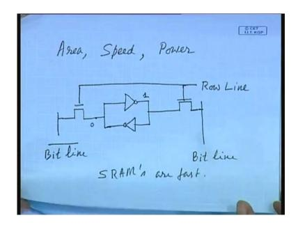
The way it is realized is,2 invertors connected, are connected back to back, then you have got 2 transistors. And when this is connected to what is known as row line and these are connected to what is known as bit line and this is bit line bar okay. So, this is bit line and bit line bar. Now, in this case you can see, there are 2 invertors connected back to back.
