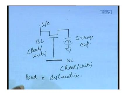
So, only 1 transistor is here and that capacitor which is explicitly fabricated is present here. This is the storage capacitor and you have got 2 or say 2 lines. This is your write line, for read and write. Watt line, for reforming read and write and this is the bit line. This is also used for read and write. So, this is watt line, this is the bit line. How it works? So, suppose the bit line is 1, you have to store 1 and then whenever you activate
