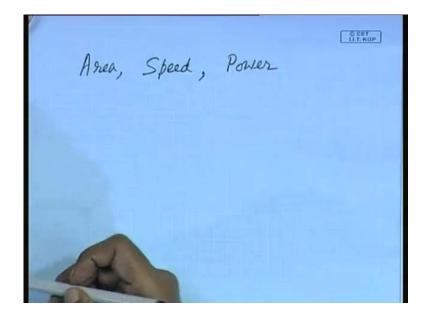
How much chip area it occupies? Then speed. How fast it is? Which is usually specified in terms of access time and the power, power dissipation is also very important in the present day context.
