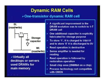
So, this is the significant improvement in the DRAM evolution, by switching to this 1 transistor dynamic RAM cell. So, only 1 additional capacitor is explicitly fabricated for storage purpose, in addition to single transistor. To store one, we charge to Vdd minus Vt. So, you are not charging to v t because, since it charge to this transistor, as you know there will be voltage drop of Vt. So, you will get Vdd minus Vt here and that will it will
