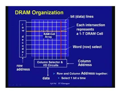
And this is the typical organization, here also you have got row decoder, column selector and I/O circuit and at the intersection you have got 1 cell, 1 transistor cell and this are the words lines and this are the column lines. And here you get data, so row and column and
