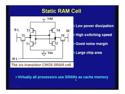
So, these are the different categories. So, we shall start with static RAM. Static RAM, basic organization of static RAM or that are the basic cell or a particular bit can be stored using the, using a, I mean bit can be stored in a cell, the organization is somewhat like this.
