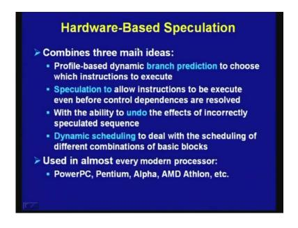
And essentially, this hardware based speculation combines three ideas, the three ideas are number 1 is profile based dynamic branch predication, to choose which instruction to execute. So, you will be using some profile based prediction technique, may be that correlating predictor or tournament predictor, some subsequent prediction technique, to choose which instruction to execute, then speculation to allow instruction to execute even before control dependences are resolved.
