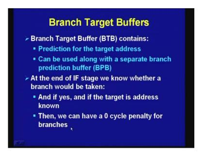
So, branch target buffer contains prediction for the target address can be used along with a separate branch prediction buffer. And, at the end of instruction fetch stage we know, whether the branch would be taken and if yes, and if the target is address known; then we can have 0 cycle penalty for branches as I elaborated in detail.
