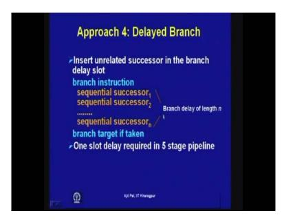
Now, we shall focus on the forth approach that is delayed branch we have seen we have a branch instruction.. Following that there are several sequential instructions and this is the target address where the, if the branch is taken it jumps to this address. So, in between the successive instruction there is a I mean and branch target address branch target if the instruction branch is taken you have got several instructions. So, these are known as sequential success of the branch instructor.
