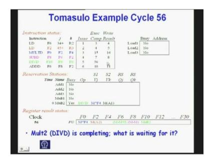
Another 1 clock cycle. So, execution is now complete and it will perform the write writing into the appropriate register that is an F 10 it will write multiplication 2 that hardware you will write.
