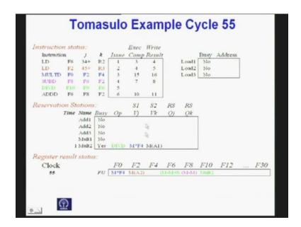
So, it will complete in and you have come to clock cycle 55. So, in clock cycle 55 we can see this division operation will require 1 more clock cycle to complete.
