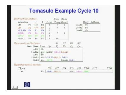
Here this is instruction execution is complete as you can see it is the time is 0. So, execution has been completed by getting the operands from the registers V j and V k. So, V j and V k have provided the operand values and the, this operation has been performed. And it will now be written into the F 6 register in the next cycle.
