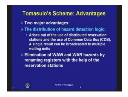
So, these are the 2 major advantages the distribution of hazard detection logic you have seen ah arises out of the use of distributed reservation stations. And the use of common data bus a single result can be broadcasted to multiple functional units and elimination of WAW and WAR hazards by renaming registers with the help of the reservation stations. So, without registers renaming has been done with the help of reservation stations by writing the values into the registers.
