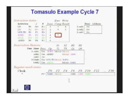
And now this instruction execution has been completed and as it is shown here that timer value has become 0. And operands are available it will write in the appropriate register that is your F 8 it will write in a F 8. So, ADD 1 adder 1 will write in F 8 that is begin and shown here and as we go to the so this instruction is completing.
