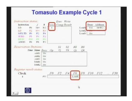
Now, we have started the clock this is the clock cycle 1 and instruction 1 has been issued. And accordingly it is a load instruction that load 1 unit has become busy. And the fetched the address be calculated is 34 plus the content of R 2. So, that will be I mean actually
