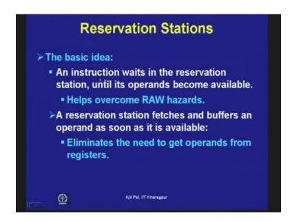
Now, let me highlights some of the important features of different functional units reservation stations single entry buffer at the head of each functional unit has been replaced by a multiple entry buffer. We have seen in case of scoreboarding there was multiple entry buffers and here it is here you have got simple single entry buffer as you can see and which are stored in the reservation stations.
