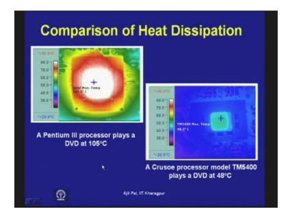
But the main benefit that you get from this VLIW processor is demonstrated by the help of this diagram. You can see here you are running the same programme one in case of Pentium 3 which is playing a DVD player. And you can see the temperature profile the Intel inside, Intel the temperature is reaching 105 centigrade. It is getting heated on the other hand in case of Crusoe processor model we find that that is you TM s 5400 playing the same programme your temperature is only 48.2.
