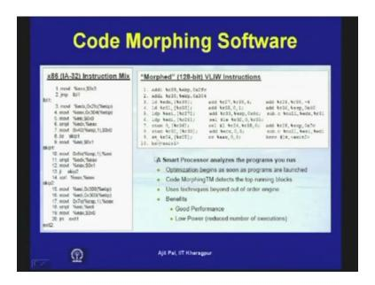
It does the forming the, that translates into VLIW codes. So, here this is the output; this is the Intel X86 instructions and this is the morphed version of the VLIW instructions. So, this is how it is being done so.
